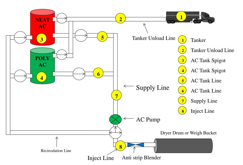
Sample at closest point to the mix - at Injection Line
