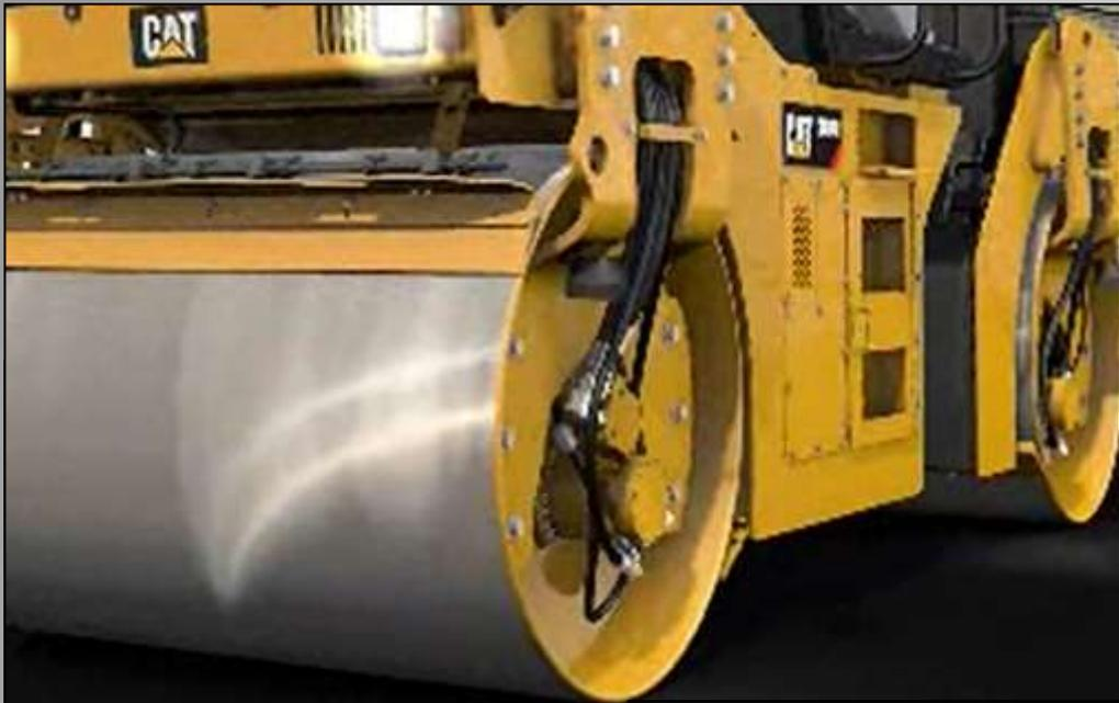
Accelerometer based technology measures deeper than the freshly laid lift of asphalt.
