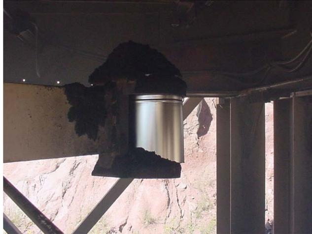
Figure 5. Mechanical tube sampling device.
