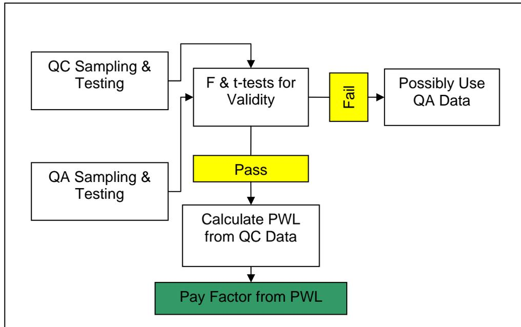
Figure 1. Components of a statistically-based quality assurance specification (after Hand and Epps 2006).
