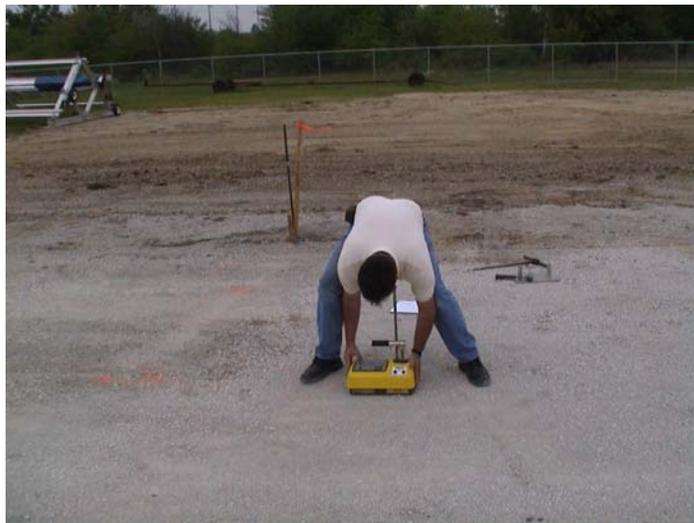
Figure 10. Nuclear density test on reconstructed aggregate subbase.
