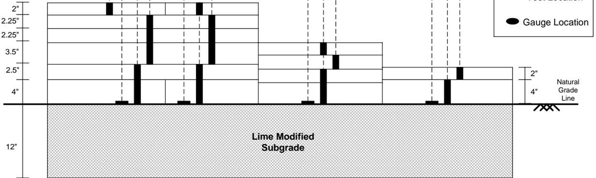
Figure 32. Coring and density locations for Lane 2.
