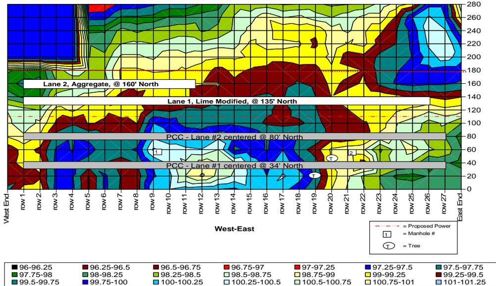
Figure 3. Topographic map of ELHMAP construction site.
