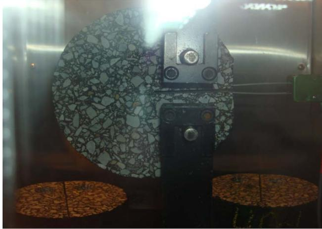
Figure 18. DCT test.
