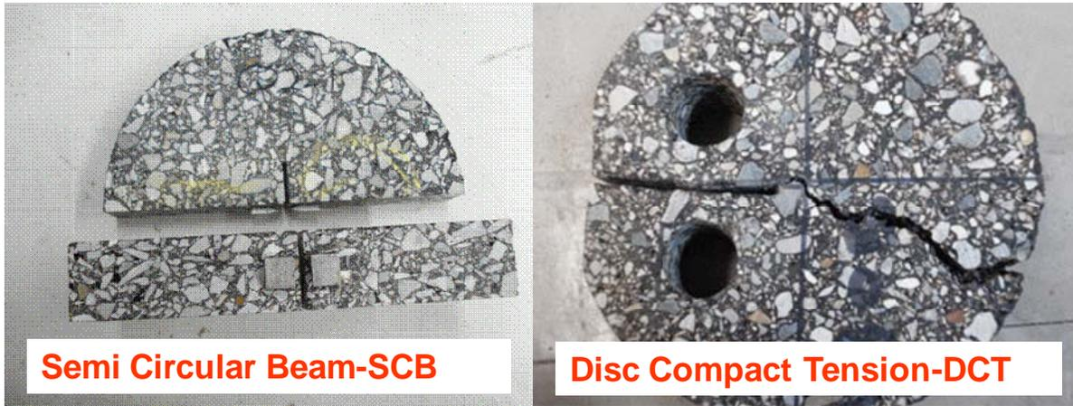
Figure 16. SCB and DCT test specimens.
