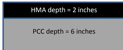
**Figures 8. 6 inch PCC with a 2 inch overlay composite pavement**
