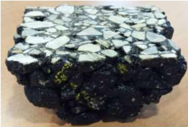
Fig. 6 - A chunk of bioasphalt
