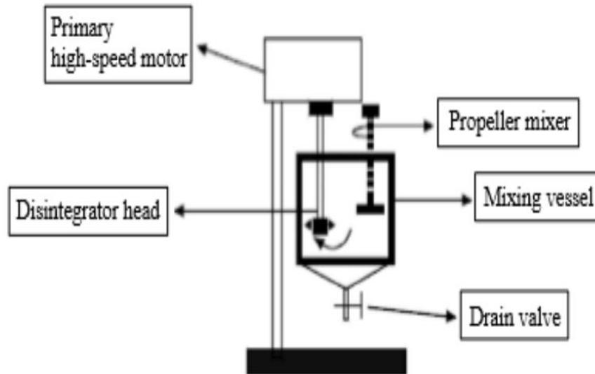
[Figure 3: Polymer-bitumen mixing assembly](#)
