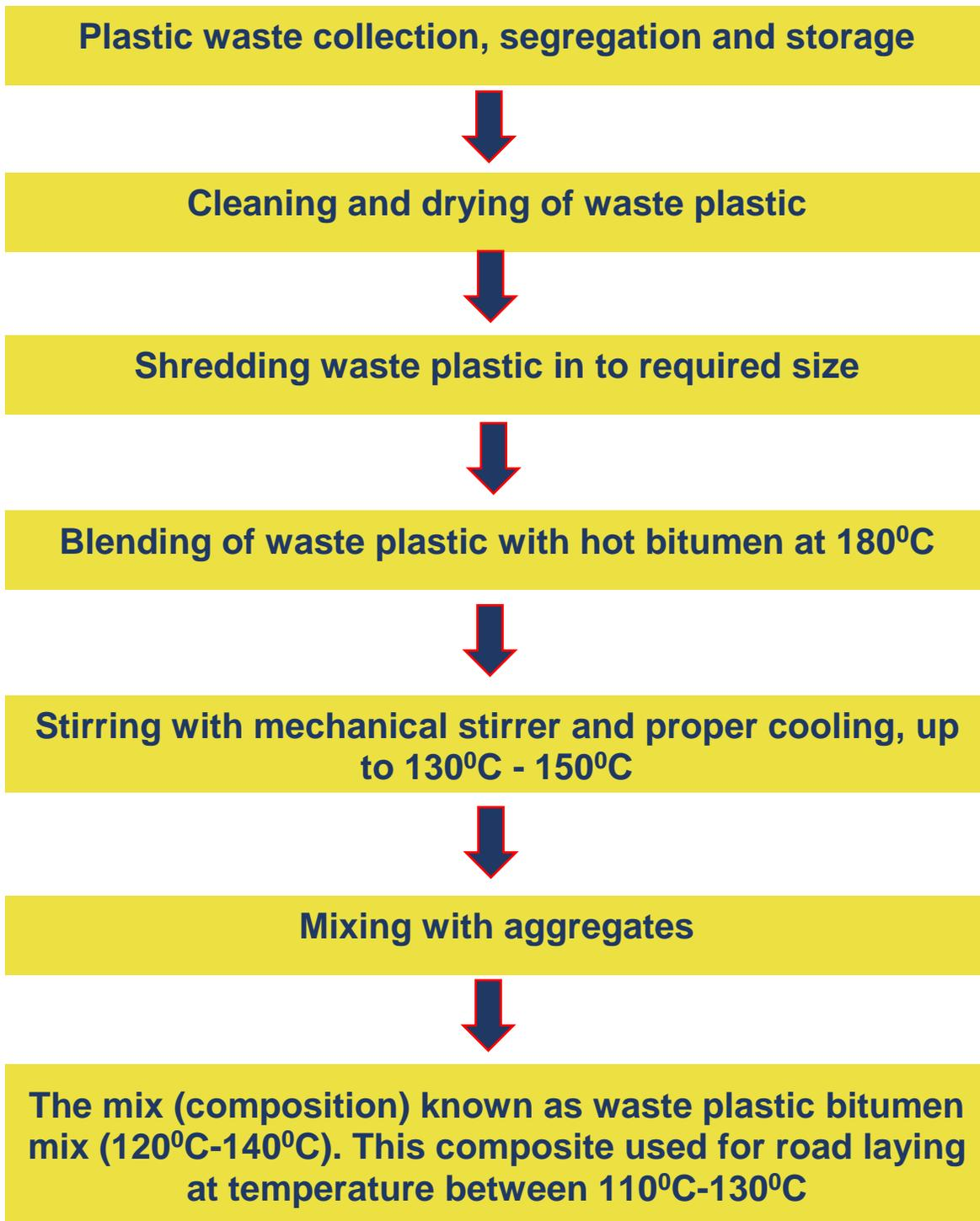
Figure4: Schematic flow diagram wet processes in reference to Dhundalwar, et al. ([2017](#))
