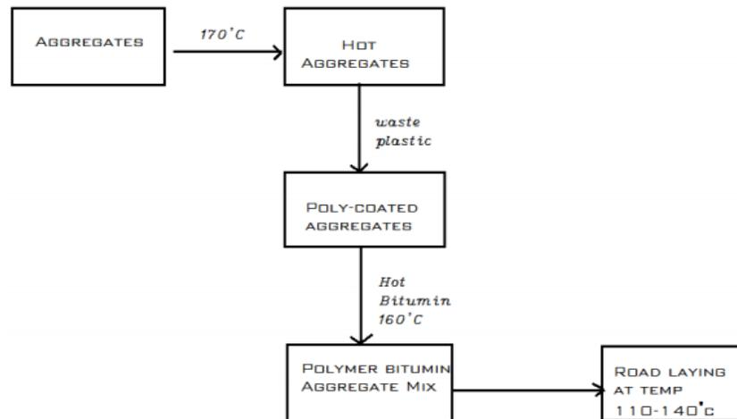
[Figure 8: Flow chart of plastic coated bitumen mix](#) from Mir, A. H. (2015)
