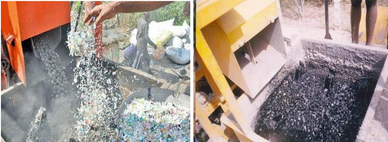
[Figure 7: Mixing of plastic and aggregate at mixing chamber](#) from
