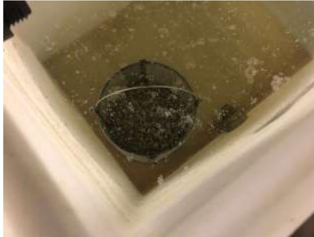
**FIGURE 9: Coarse Aggregate Specific Gravity Water Weight Determination**
