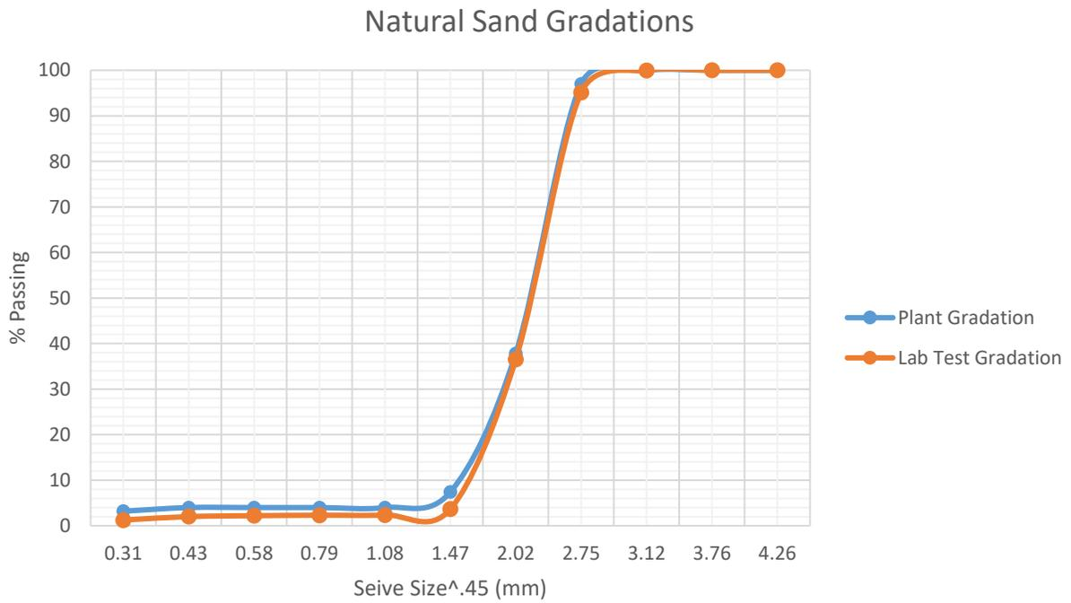
**FIGURE 6: Natural Sand Gradations (Fine Aggregate)**
