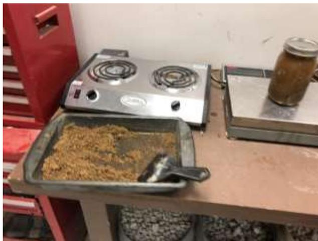
**FIGURE 12: Fine Aggregate SSD Condition**
