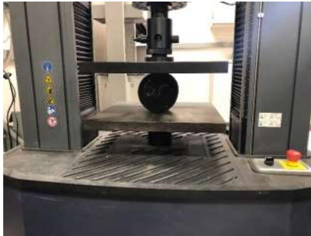
**FIGURE 18a: Creep Test in Progress.**
