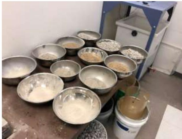
**FIGURE 13: Aggregate Proportioning**
