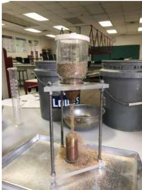
**Figure 8: Uncompacted Voids Apparatus**
