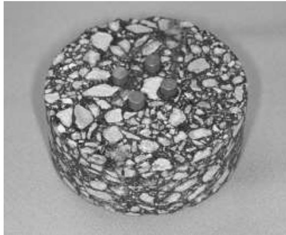
**Figure 2: Prepared Sample with Gauge Points (Protocol P07 2001)**
