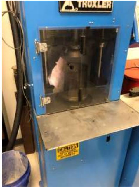
**FIGURE 16: Sample Compaction**
