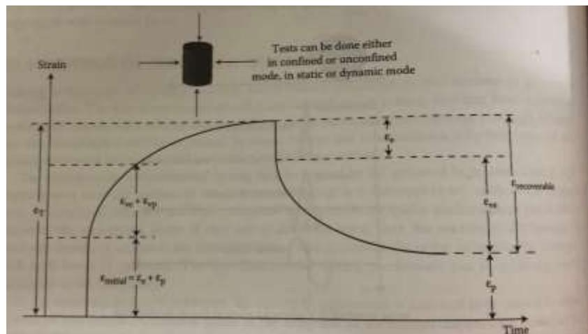
**Figure 4: Schematic of Creep Testing (Mallic El-Korchi 2013)**
