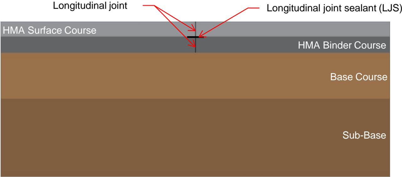
**Figure 12. Section of roadway with LJS installed.**
