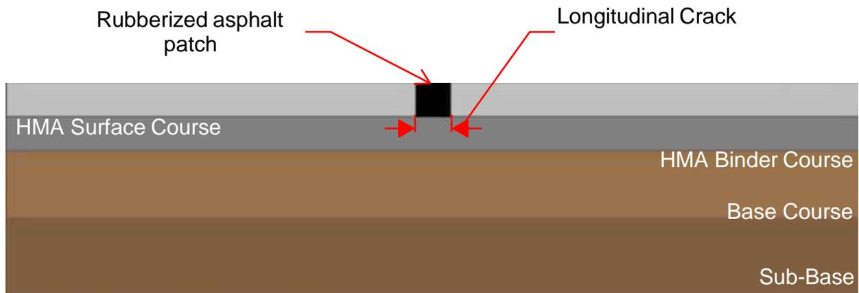
**Figure 9. Section cut of a repaired crack.**
