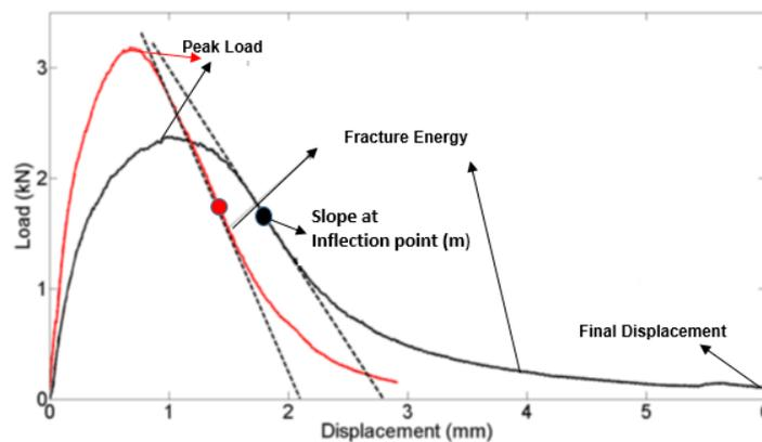
**Figure 2. Typical IFIT Output Showing Important Parameters.**
