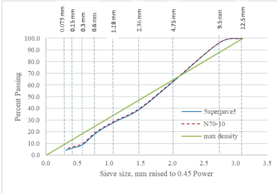
**Figure 1. Aggregate Blend Gradations for the Two AC Mixes.**
