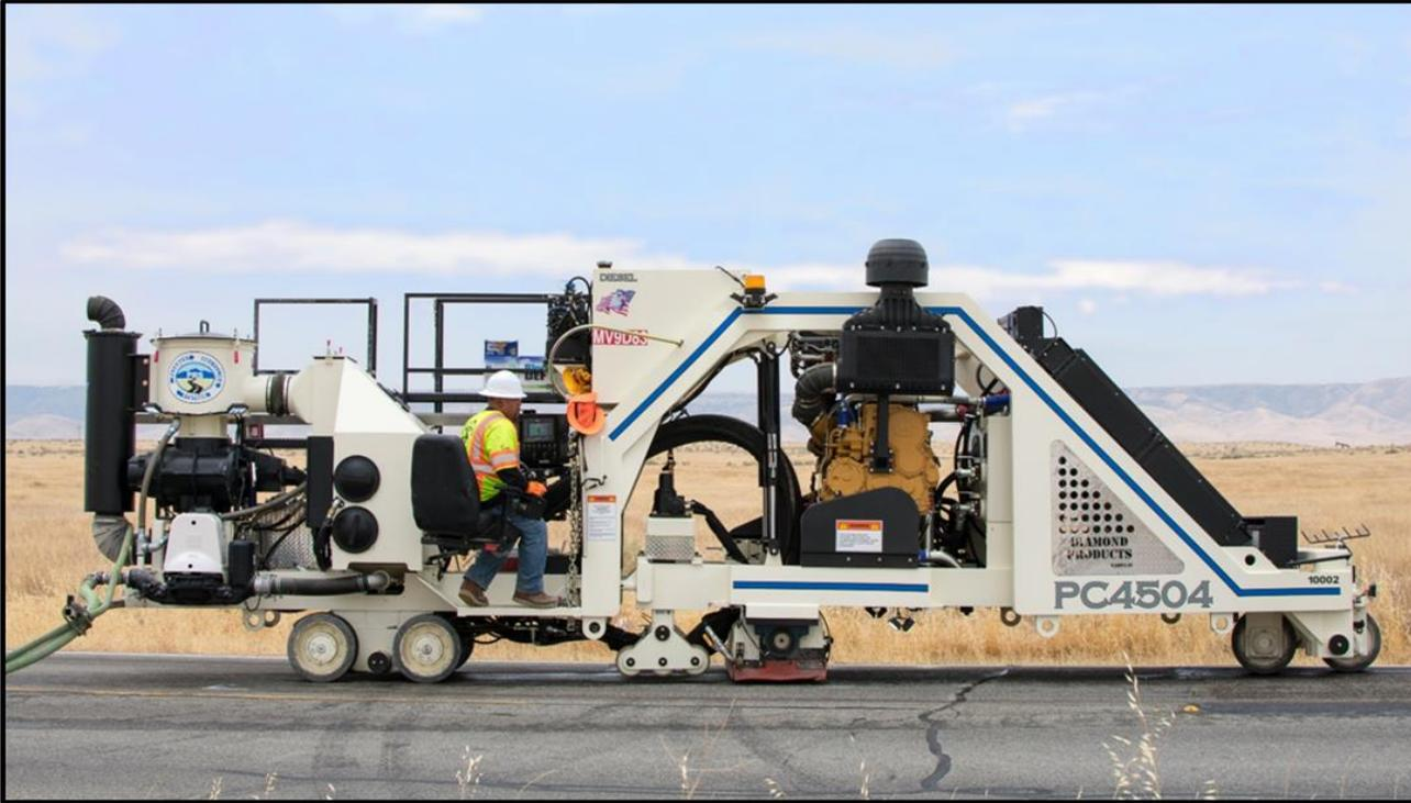
Is a "rigid" frame planer equipped with diamond tipped blades
