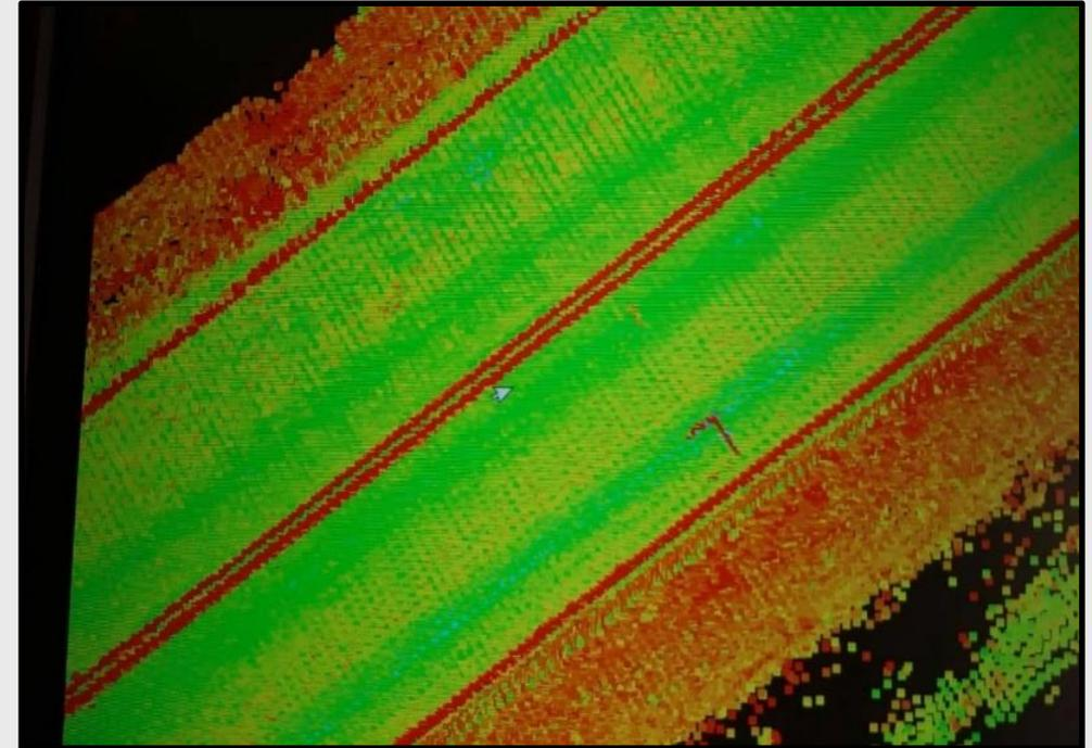
Uses GPS to Position Horizontally with Scanned Surface for Vertical Road Surface
