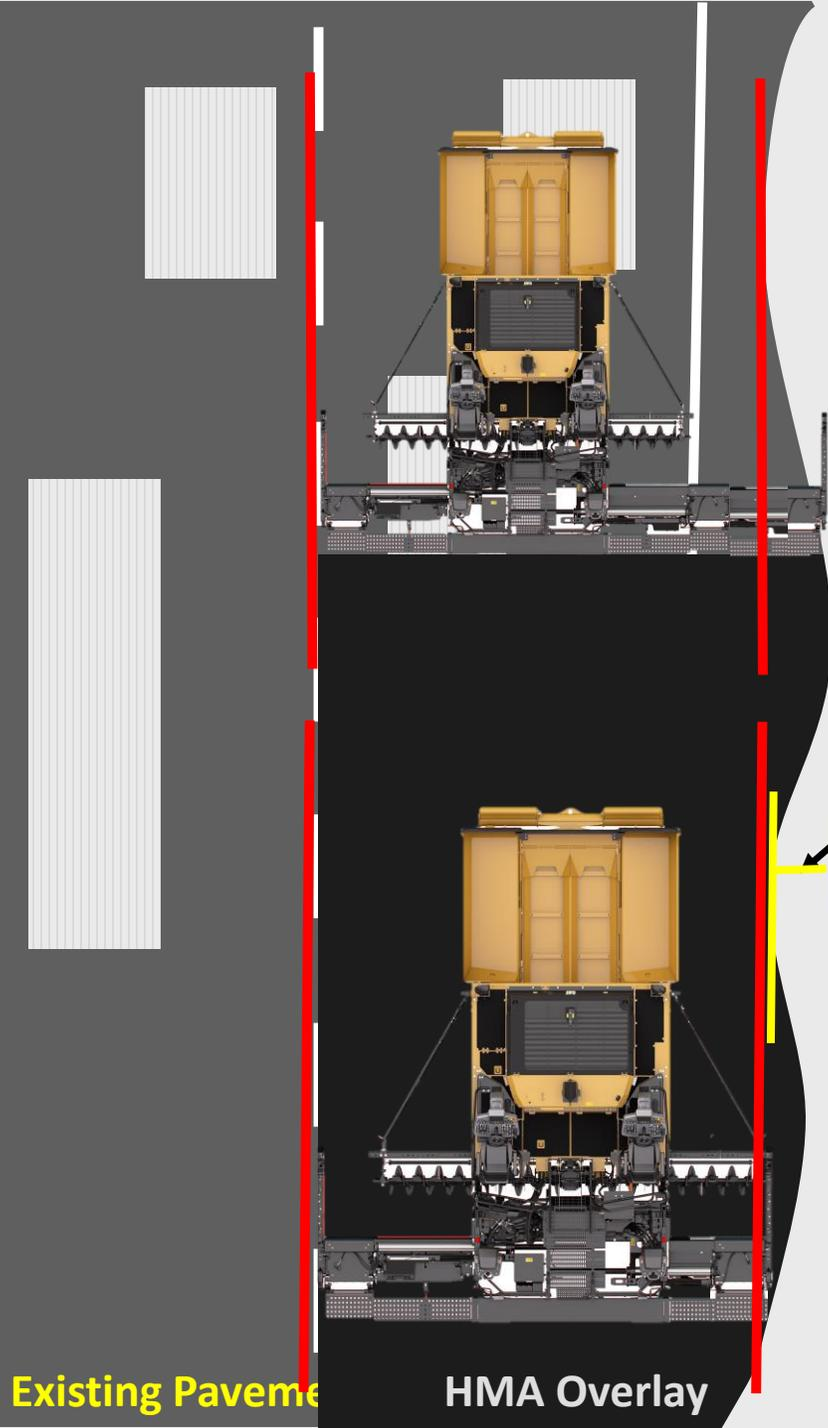
Variable width paving causes a change to the head of material against the screed
