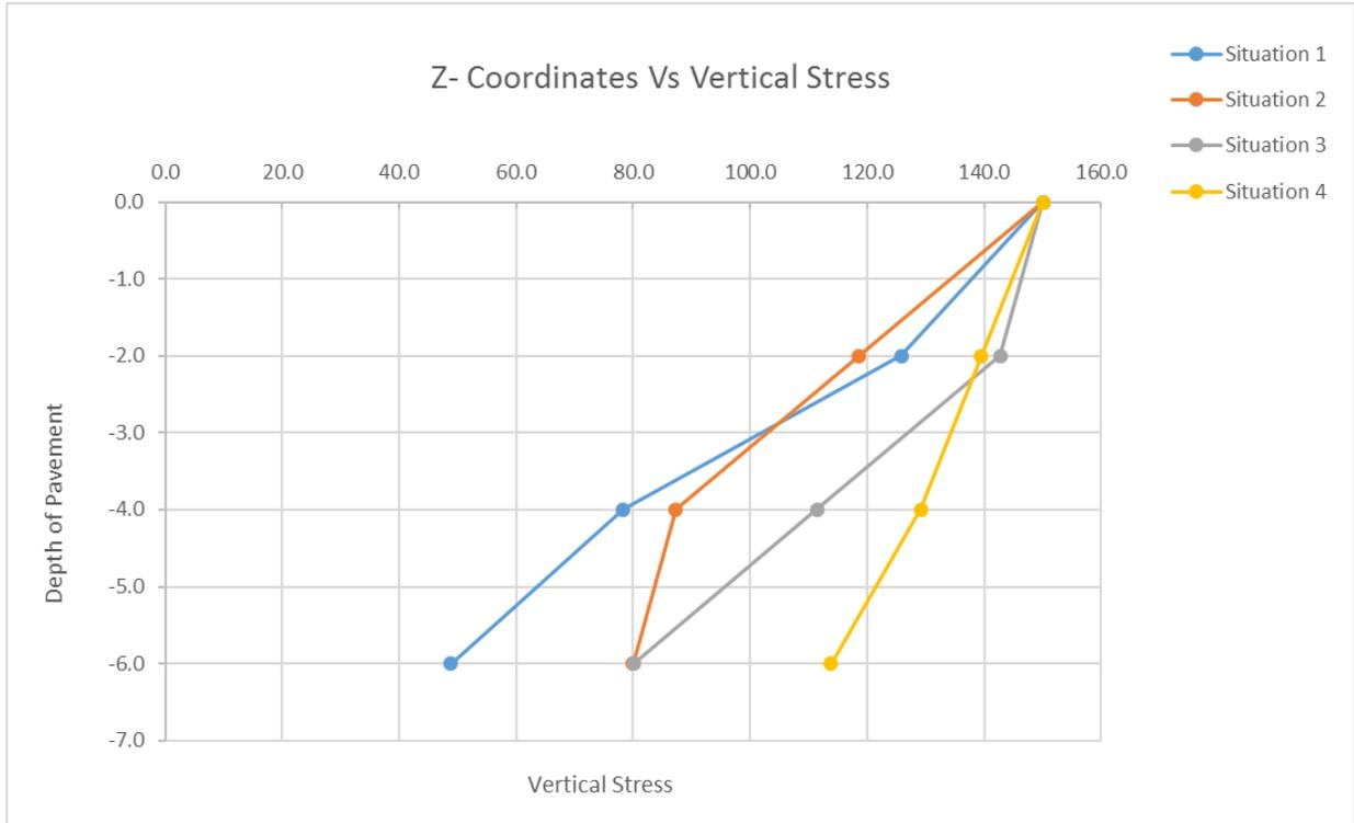
**Figure 4.** The relationship between the layers and the vertical stress for the four different interface conditions.
