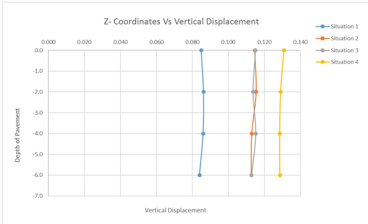
**Figure 5.** The relationship between the layers and the Vertical displacement for the four different interface conditions.
