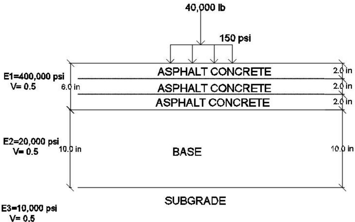
**Figure 1.** Asphalt concrete pavement layers under a wheel load.
