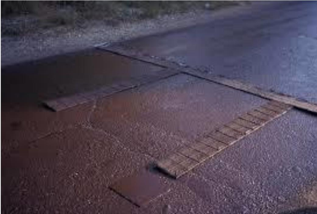
Figure 5. Weighing pads used to see how much tack coat has been applied [5]
