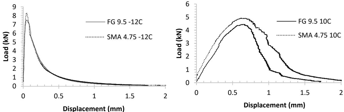
Figure 2 SCB load-displacement curve for mixes FG 9.5 and SMA 4.75: (Left) Load-CMOD curves at  $-12^{\circ}\text{C}$ , (Right) Load-LLD curves at  $10^{\circ}\text{C}$ .
