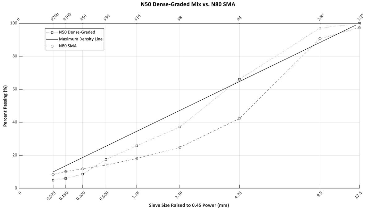
**Figure 2: 0.45 Power Gradation Chart showing mix comparison.**
