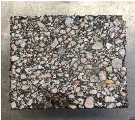
**Figure 3: 9.5 NMAAS SMA Section.**
