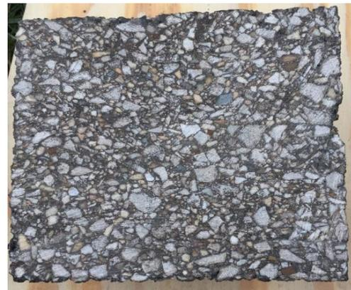
**Figure 4: 9.5 NMAAS Dense-Graded Mix Section.**
