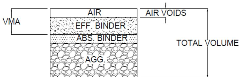
**Figure 1. HMA Volumetric Diagram.**
