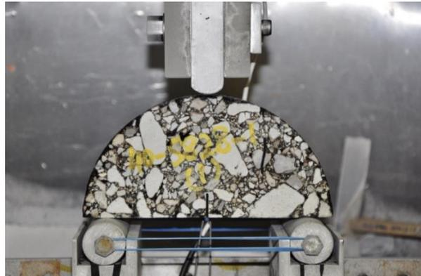
Figure 2. A specimen in the Semi-Circular Bending Test (Al-Qadi et al., 2012).
