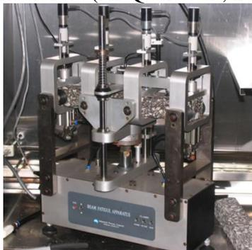
Figure 3. A Specimen in the Beam Fatigue Test (Flexural Fatigue, 2018).
