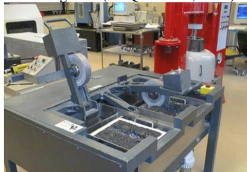
Figure 4. Specimens in the Wheel Tracking Test (Stuart et al., 2001).
