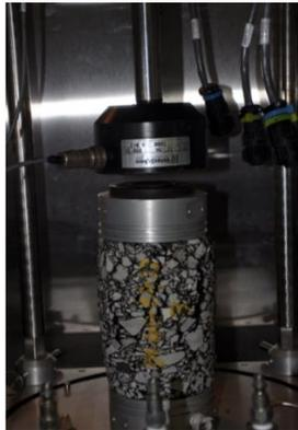
Figure 1. A Specimen in the Flow Number Test (Al-Qadi et al., 2012).
