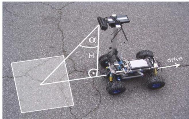
Figure 6. shows a remotely controlled sensing Robot vehicle for the experiment (Koch *et al.*, 2013)
