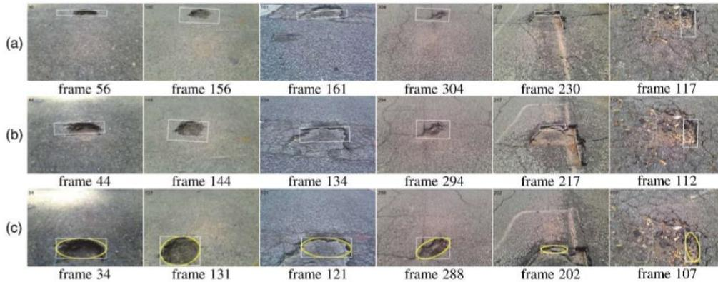
Figure 5 . shows selected potholes-recognition results in pavement videos (Column by Column) (a) tracking results; (b) tracking results; (c) detection results (Koch *et al.*, 2013).
