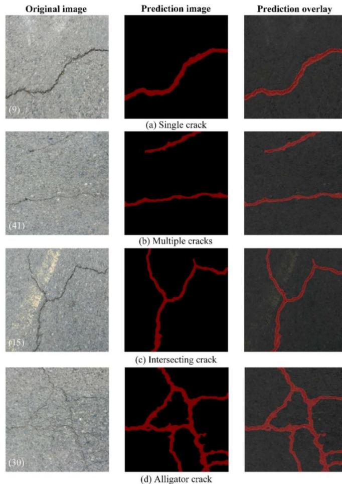
Figure 7. shows test results of four types of cracks in asphalt pavement (Ji *et al.*, 2020).
