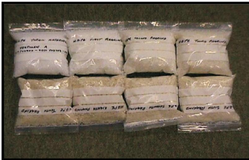
Figure 1. The color change in HDPE can be clearly seen after 10 process cycles. Virgin material (top left), material injection molded, and re-granulated 10 times (bottom left).
