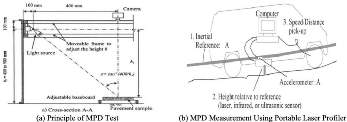
Figure 2. Measurement Principle of Mean Profile Test Using Portable Laser Profiler (Kim et al., 1579)
