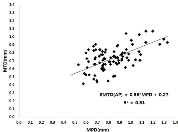
Figure 3. Correlation of Sand Patch Test and Portable Laser Profiler (Kim et al., 1586)
