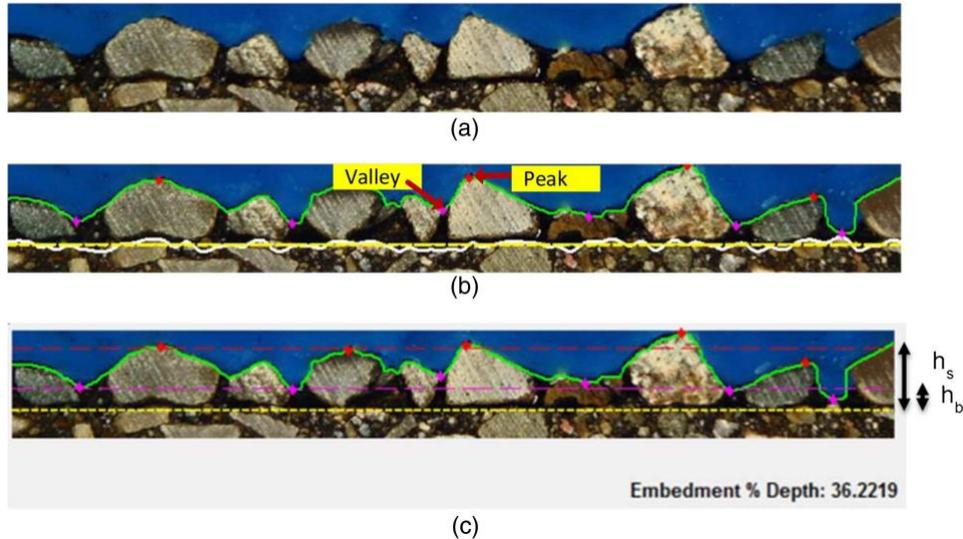
Figure 9. Steps of the peak and valley method: (a) original image; (b) finding peak and valley points—existing pavement’s determination; and (c) embedment depth calculation (Ozdemir et al.)
