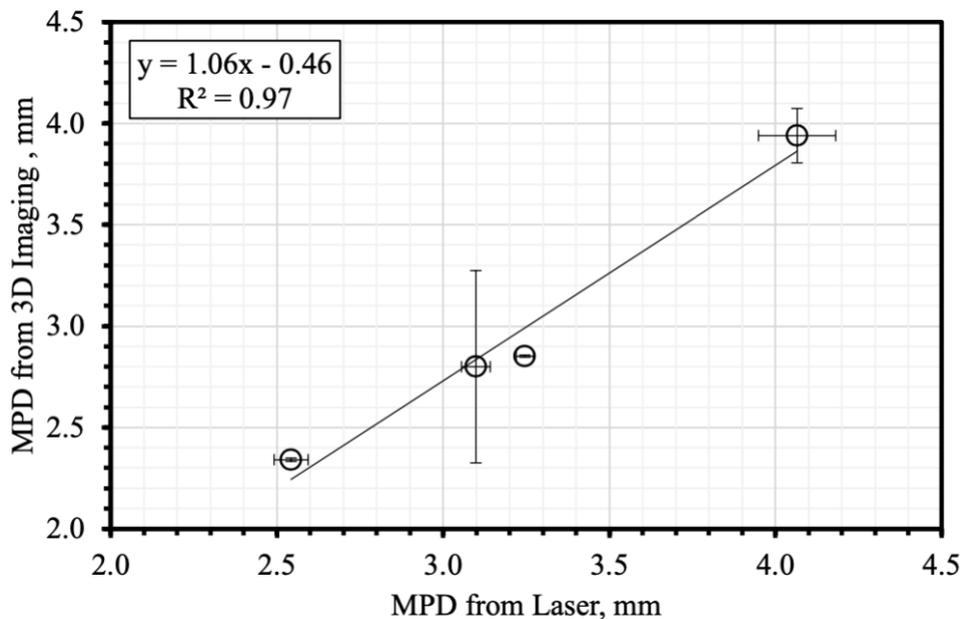
Figure 6. The Correlation Between the 3D Image-based Method and the Laser-Based Method (Boz et al., 53)
