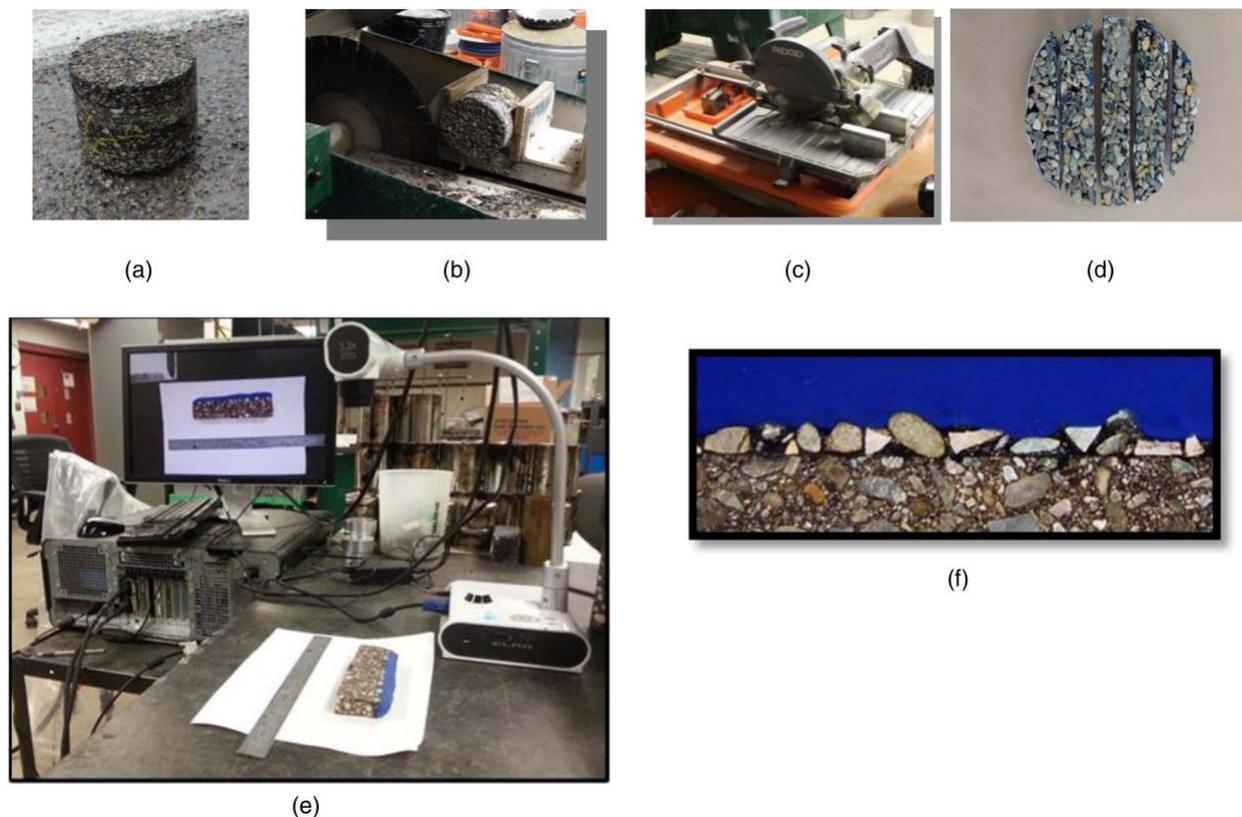
Figure 7. Preparation and picture of sample: a) coring in the field; b) horizontal cutting; c) vertical slicing; d) core slices; e) image acquisition of the core slice; f) the desired image of the cross-section (Ozdemir et al.)
