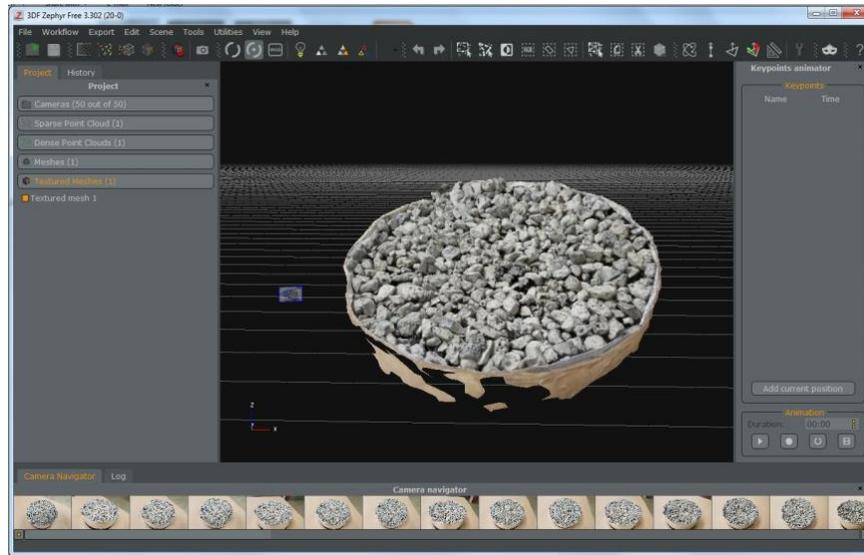
Figure 4. A 3D Model of a Chip Seal Specimen (Boz et al., 52)
