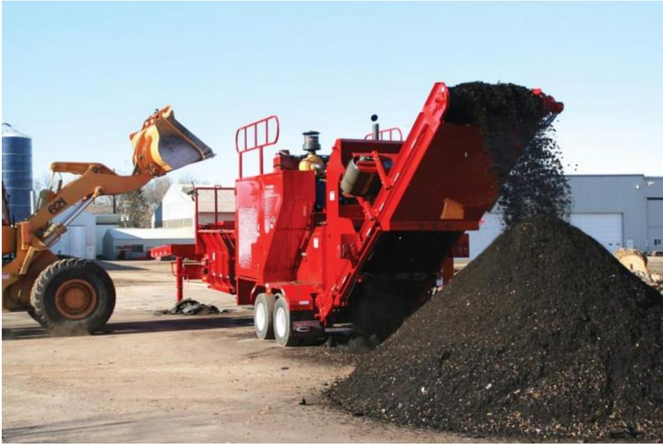
Figure 2) Shingles being grinded down (16)
