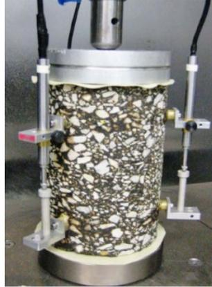
**Figure 16 Dynamic modulus test setup (Y. Zhang et al., 2012)**
