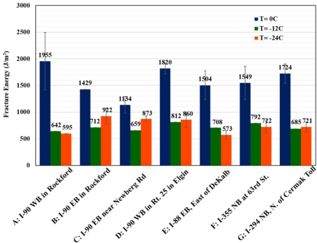
Figure 6. Fracture energy results of testing sections
