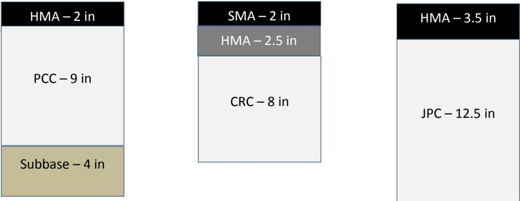
**Figure 5. Cross-section of test pavements on the following interstates in Illinois: I-94 near Gurnee, I-64 near Fairview Heights, and I-294 in Chicago respectively.**
