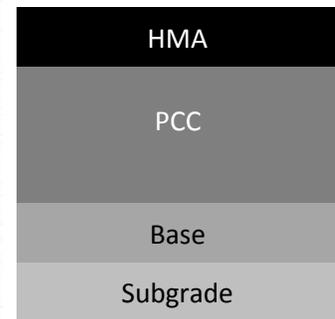
**Figure 1: Typical Cross Section Composition**
