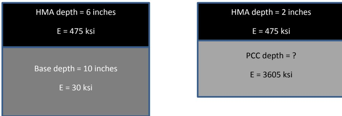
**Figure 6. Equivalent depths of HMA and composite pavements.**
