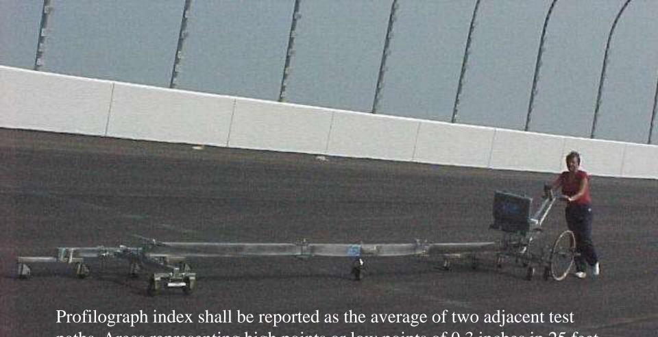
Profilograph index shall be reported as the average of two adjacent test paths. Areas representing high points or low points of 0.3 inches in 25 feet shall be corrected by the contractor. This criteria shall be met regardless of the average index of the 0.1 mile section. The maximum allowable profile index for a 0.1 mile section is 12 inches per mile equivalent over a 0.1 mile stretch for the base and leveling courses, and 8 inches per mile for the wearing course.
