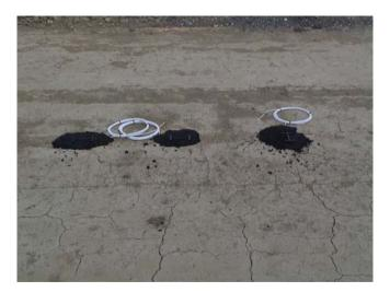
Figure 22. Placement of strain gauges.
