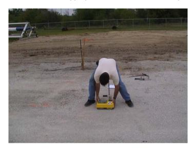
Figure 10. Nuclear density test on reconstructed aggregate subbase.
