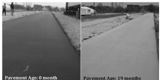
Figure 1. Pavement section at the Advanced Testing and Research Engineering Laboratory (ATREL) at the University of Illinois. Immediately after the construction (left) and 19 months after construction (right). Figure reproduced from Dave *et al*<sup>[1]</sup>
