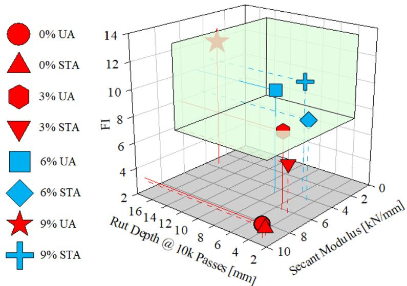
**Fig. 5** 3D Interaction plot between rut depth, FI, and secant modulus
