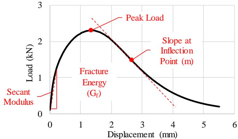
Fig. 1 Typical outcome from I-FIT test, after Ozer et al. [15]
