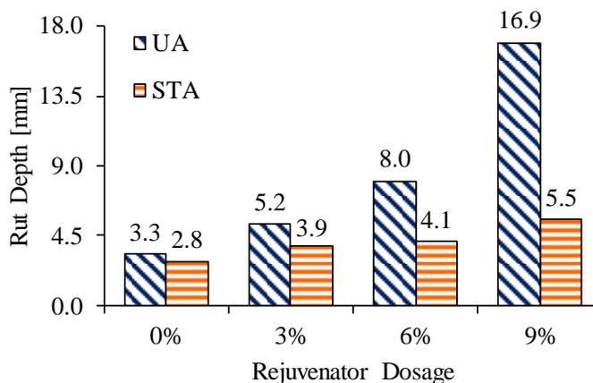
**Fig. 3** Final rut depth at 10,000 passes, all blends.
