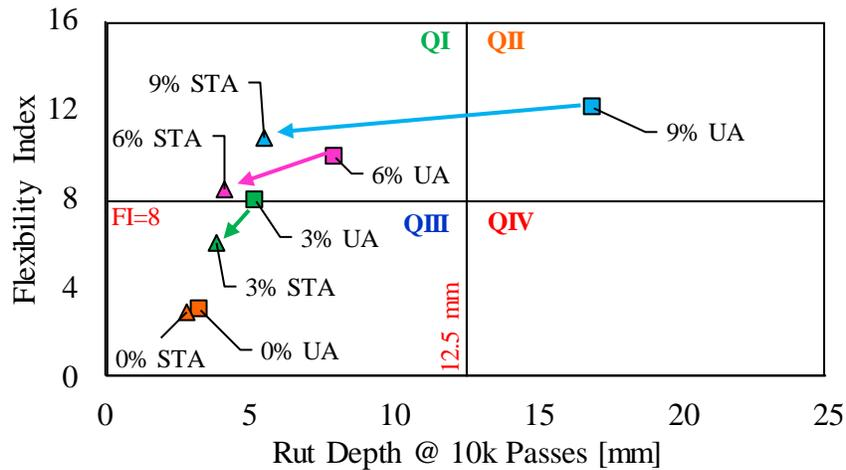
**Fig. 4** 2D Interaction plot between rut depth and FI
