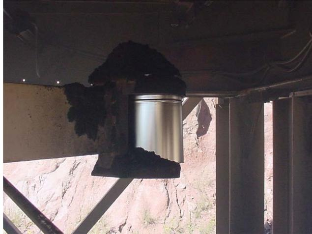
Figure 5. Mechanical tube sampling device.
