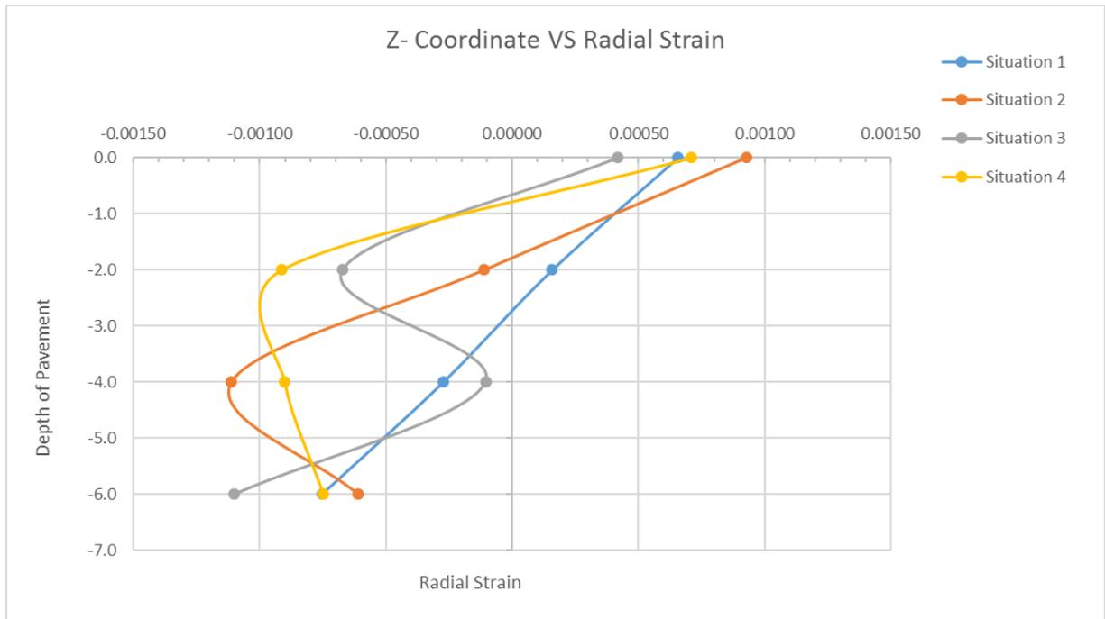
**Figure 3.** The relationship between the layers and the radial strains for the four different interface conditions.
