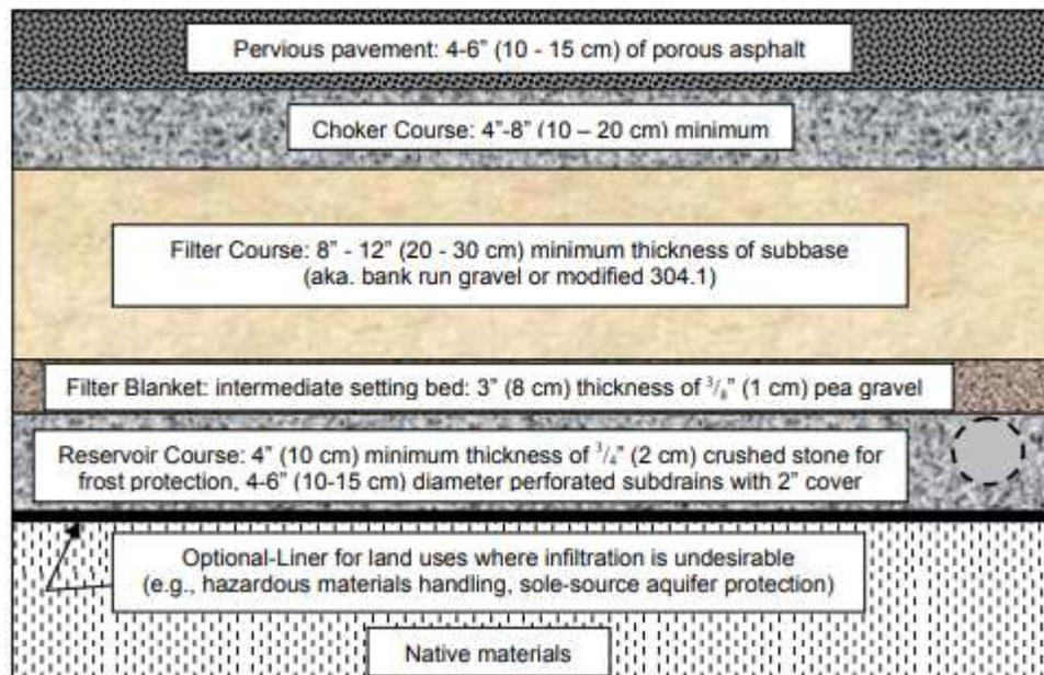
Figure 1 Cross Section of the Pavement [1]
