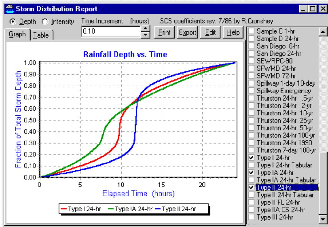
**Figure 2. Storm Distribution Report example provided from HydroCAD**
