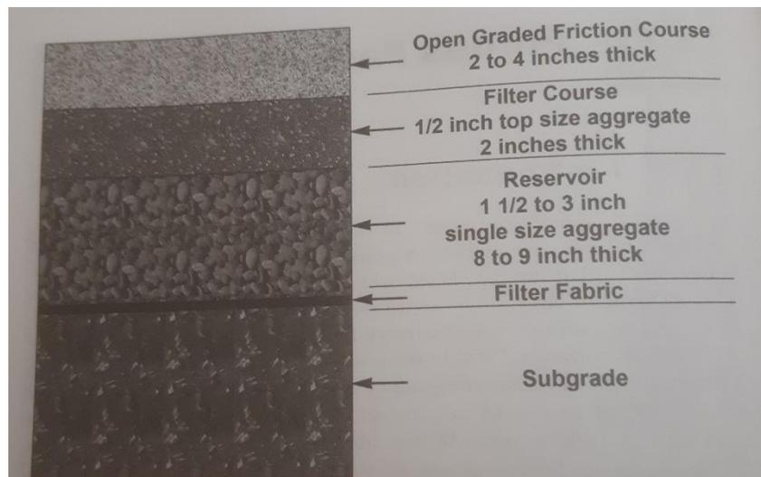
**Figure 1. Layers of Porous Pavement**
