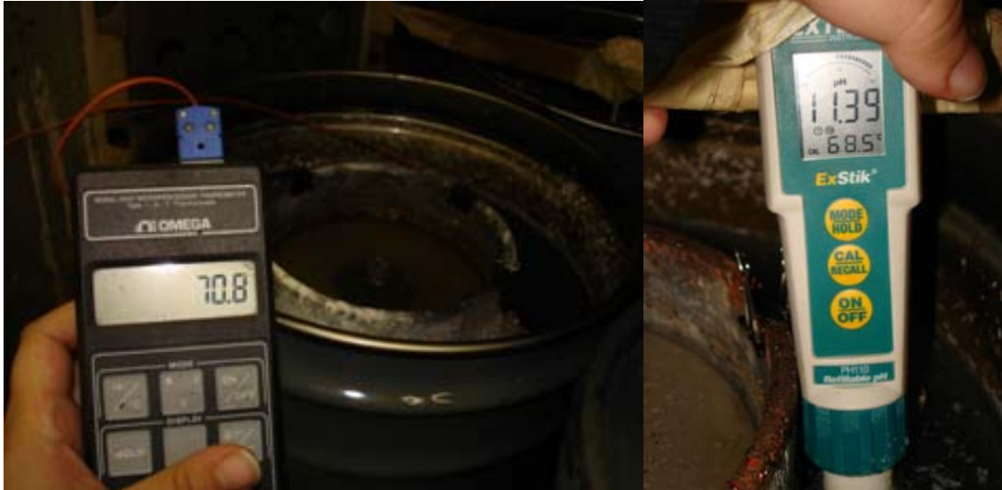
Figure 13. Photos showing daily temperature and pH measurements of the high alkali cement water solution used for soaking the specimens.
