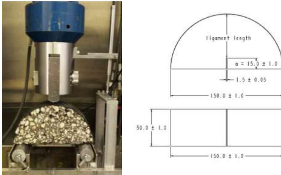
*Figure 2 SCB test fixture and configuration (left) and geometry of specimen and fixture (right) with an external linear variable differential transformer (LVDT, based on the submitted AASHTO Provisional Standard Test Method)*
