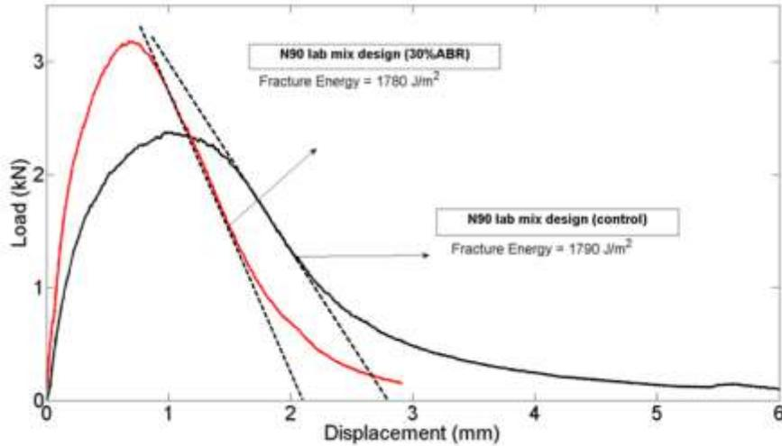
Figure 4 Major characteristics derived from load-displacement curves from IL-SCB tests conducted at 25°C (77°F) and at 50 mm/min (2 in/min) displacement rate illustrating the potential effects of ABR.
