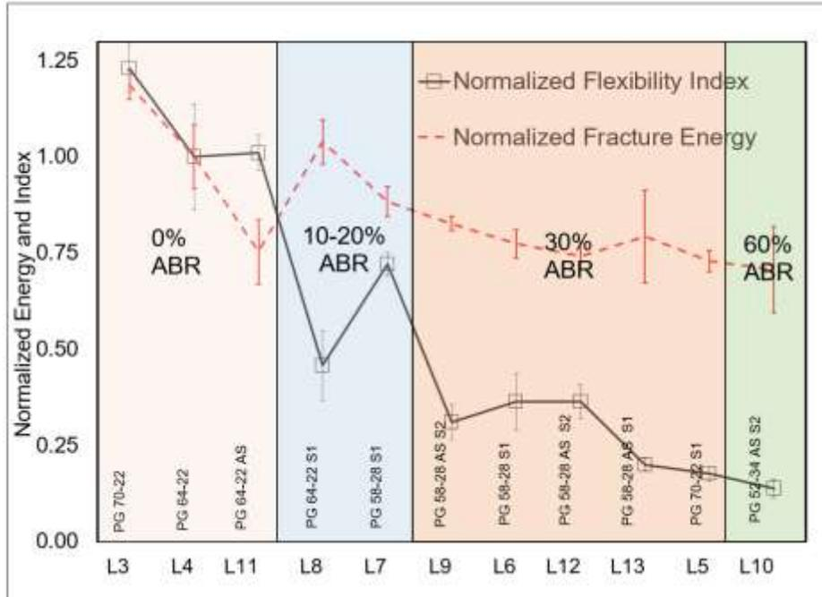
Figure 5 Normalized FI Results for the ICT Designed Plant Mixtures (FI Normalized based on mix L4)
