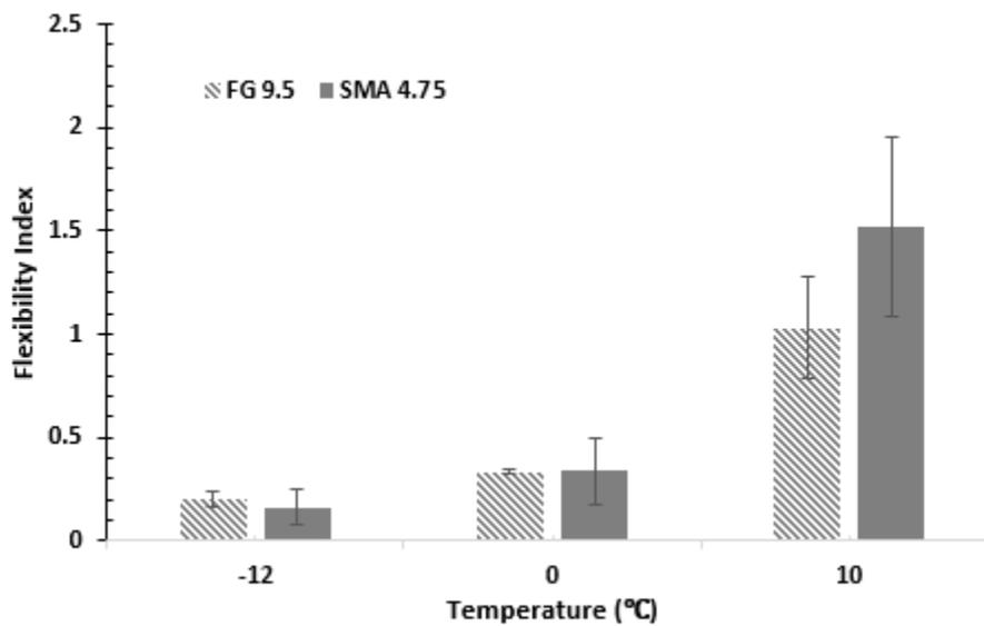
Figure 4 Flexibility index of FG 9.5 and SMA 4.75 at -12, 0, 10°C.
