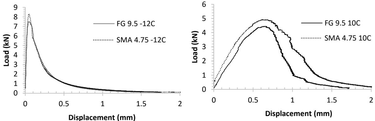
Figure 2 SCB load-displacement curve for mixes FG 9.5 and SMA 4.75: (Left) Load-CMOD curves at  $-12^{\circ}\text{C}$ , (Right) Load-LLD curves at  $10^{\circ}\text{C}$ .
