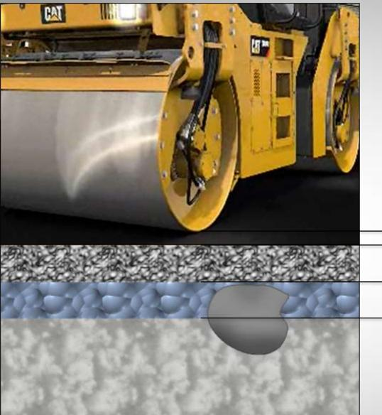
Accelerometer based technology measures deeper than the freshly laid lift of asphalt.
