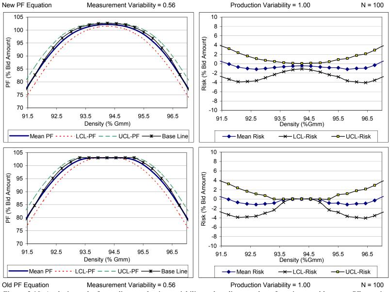
Figure. 3.10: Analysis results for medium production variability and medium number of specimens: old vs. new PF equation
