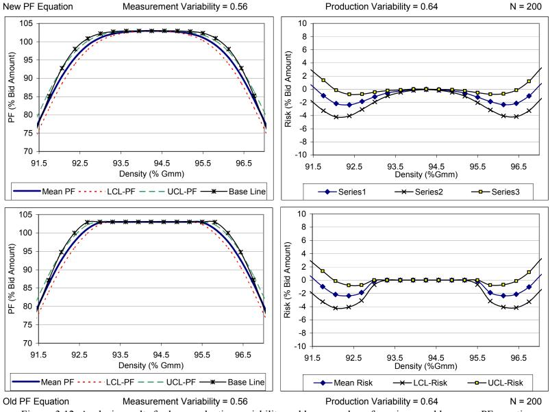
Figure. 3.12: Analysis results for low production variability and large number of specimens: old vs. new PF equation
