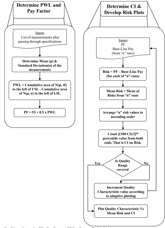
Key: CI – Confidence Interval; PF – Pay Factor; PWL – Percent Within Limit;  $N(\mu, \sigma)$  – Normal Probability Distribution With Mean =  $\mu$  and Standard Deviation =  $\sigma$
