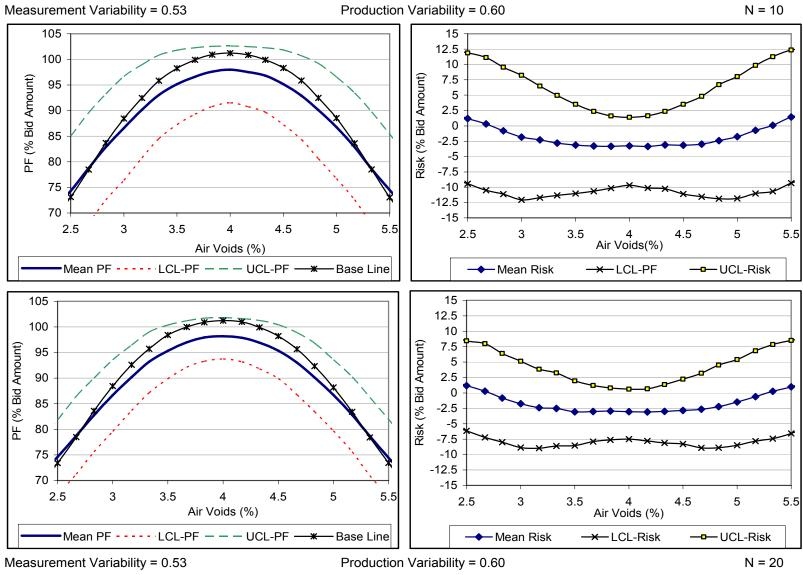
Figure 3.15: Analysis results for air voids: N=10 vs. N=20
