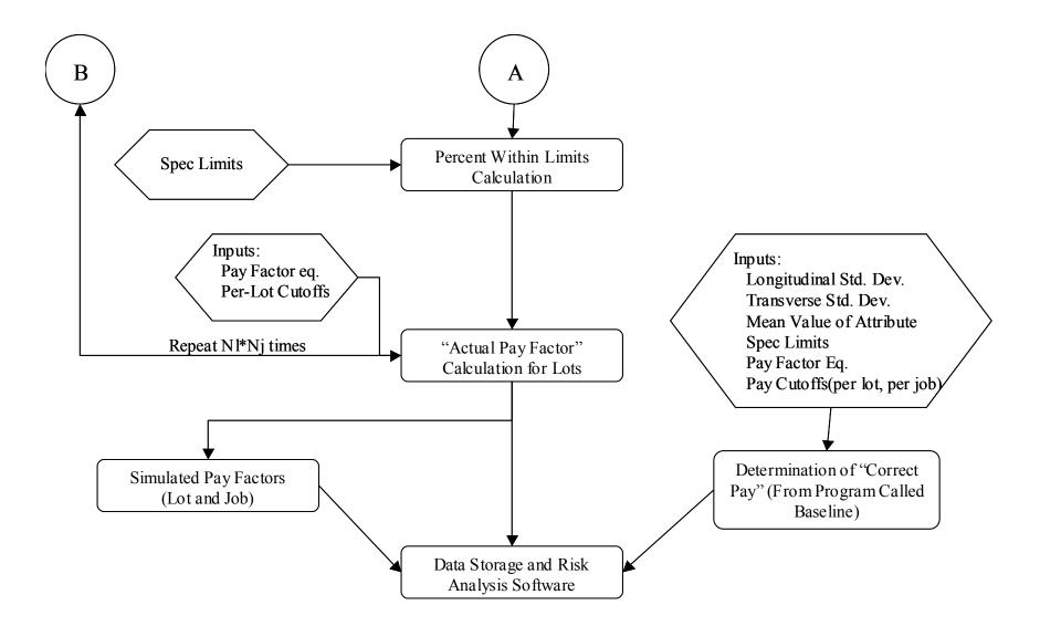
Figure A1.1b: ILLISIM program flowchart, part 2 of 2.
