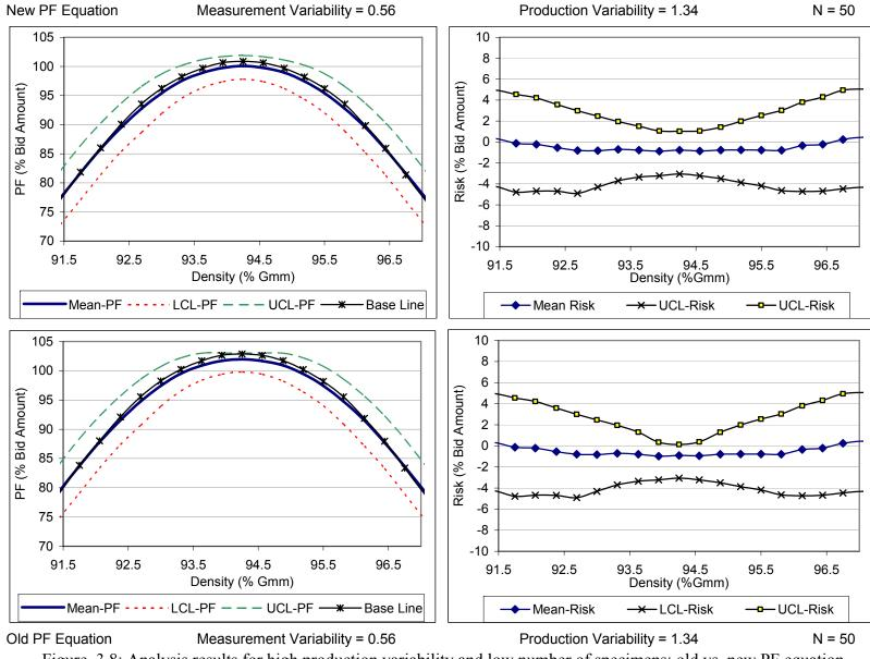
Figure. 3.8: Analysis results for high production variability and low number of specimens: old vs. new PF equation
