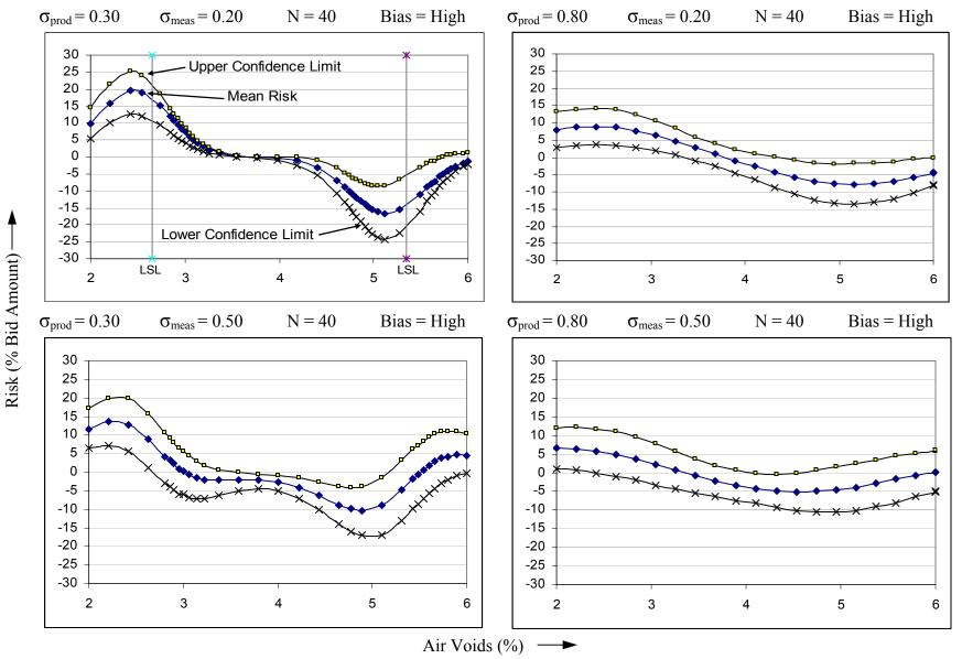
Fig 3.4: Sensitivity analysis simulation run plots from SRA (LSL, USL: Lower and Upper Specification Limits)
