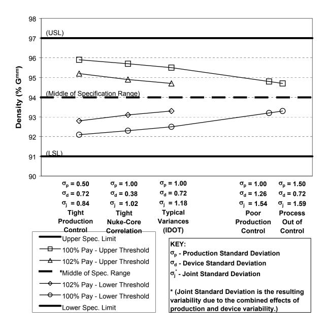
Figure A1.8: Use of ILLISIM to Determine Possible Operating Ranges as a Function of Payment Level and Combined Variability
