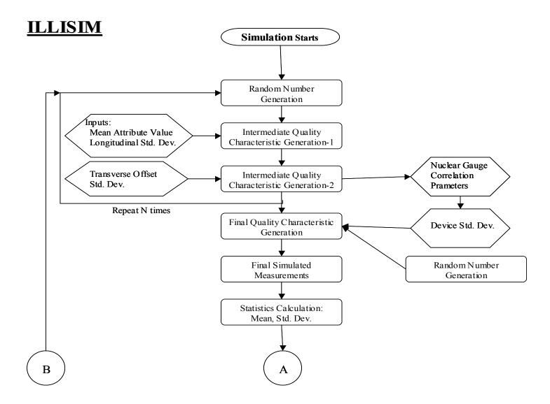
Figure A1.1a: ILLISIM program flowchart, part 1 of 2. Letters 'A' and 'B' at the bottom of the chart indicate connecting points for the ensuing figure.
