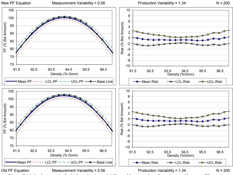
Figure. 3.14: Analysis results for high production variability and large number of specimens: old vs. new PF equation
