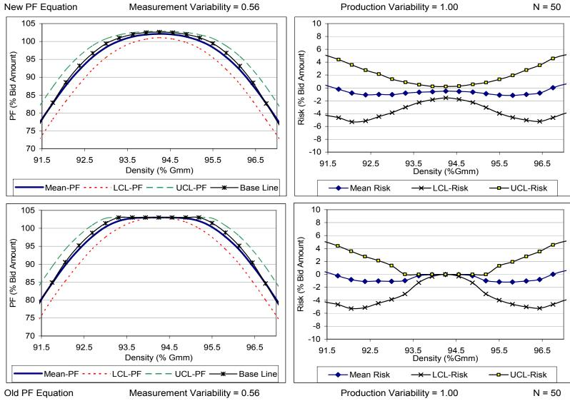
Figure. 3.7: Analysis results for medium production variability and low number of specimens: old vs. new PF equation
