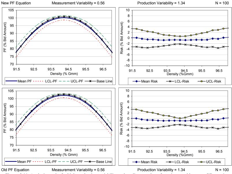
Figure. 3.11: Analysis results for high production variability and medium number of specimens: old vs. new PF equation
