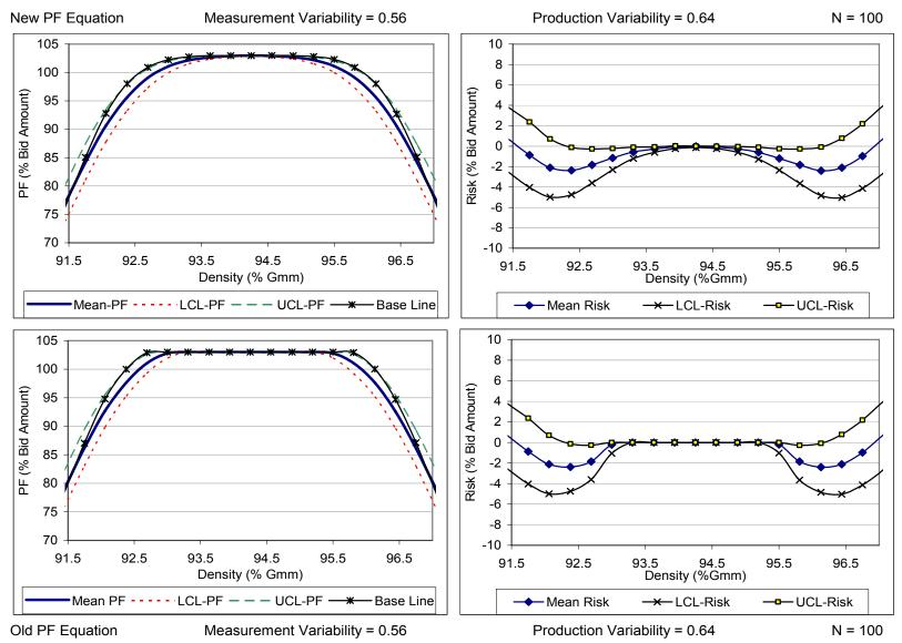
Figure. 3.9: Analysis results for low production variability and medium number of specimens: old vs. new PF equation
