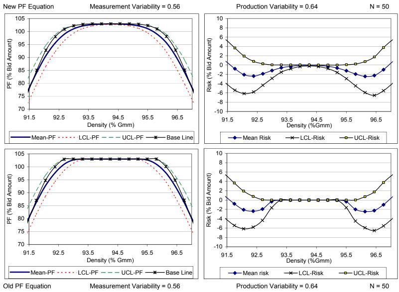
Figure. 3.6: Analysis results for low production variability and low number of specimens: old vs. new PF equation
