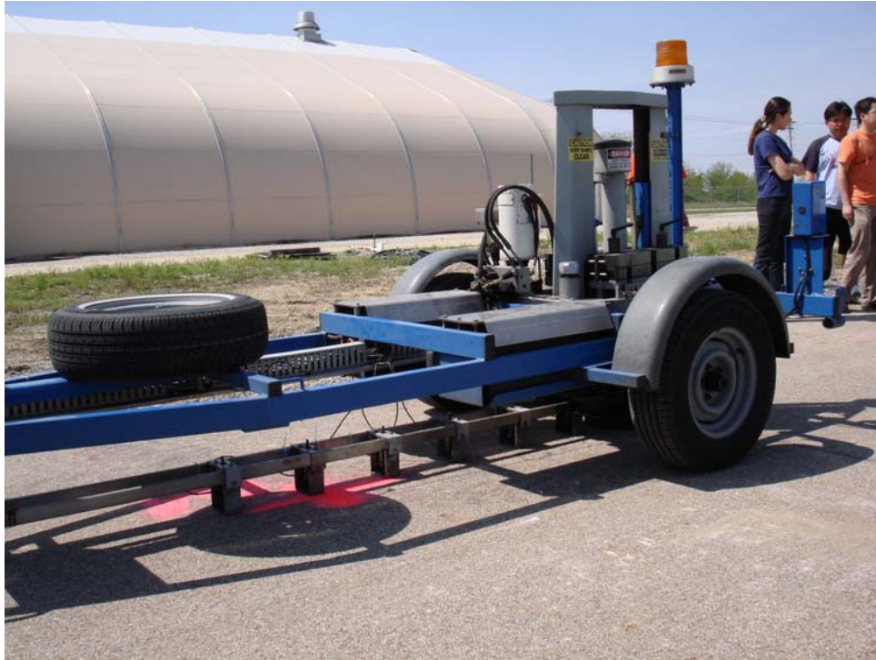
Figure 2-1. Dynatest FWD device used by IDOT.
