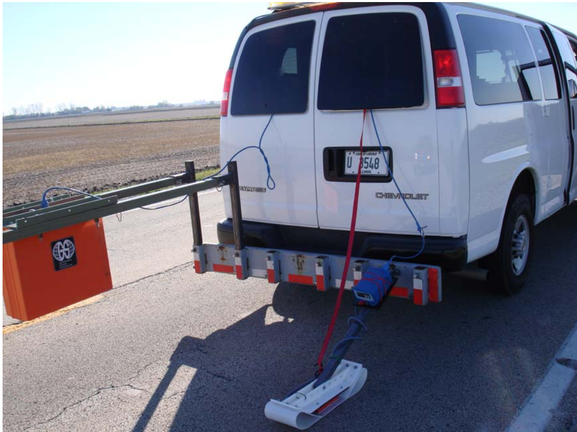
Figure 4-9. Air and ground coupled antennae used in GPR testing.
