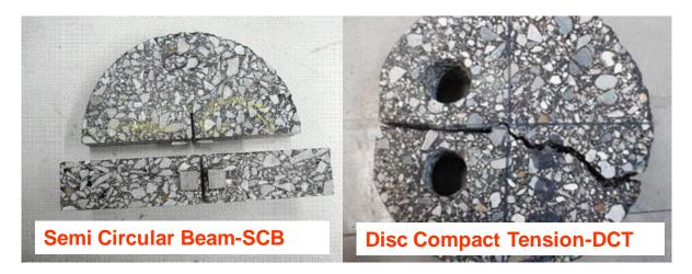
Figure 16. SCB and DCT test specimens.
