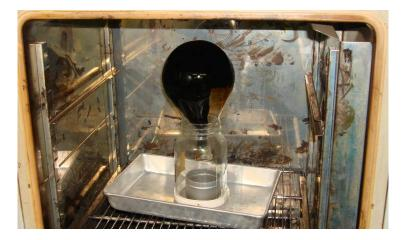
Figure 4. Binder draining from collection flask in oven.
