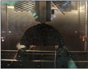
Figure 17. SCB test.
