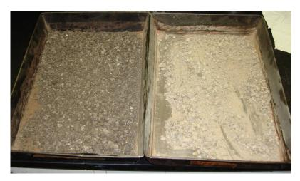
Figure 6. RAP material before (left) and after (right) extraction.
