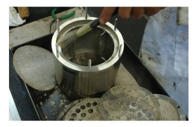
Figure 5. Brushing the extraction vessel clean of fine material.
