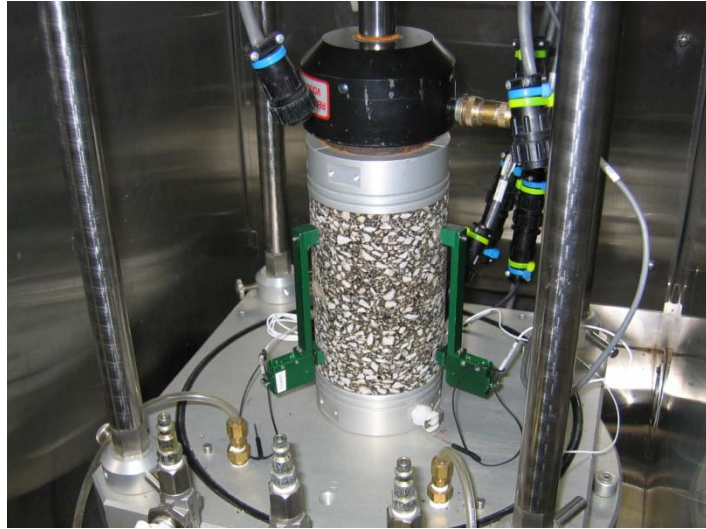
Figure 4. Dynamic Modulus Testing Setup
