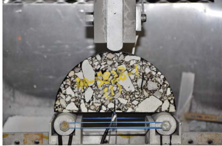
Figure 7. Semi-circular bending beam (SCB) test fixture.
