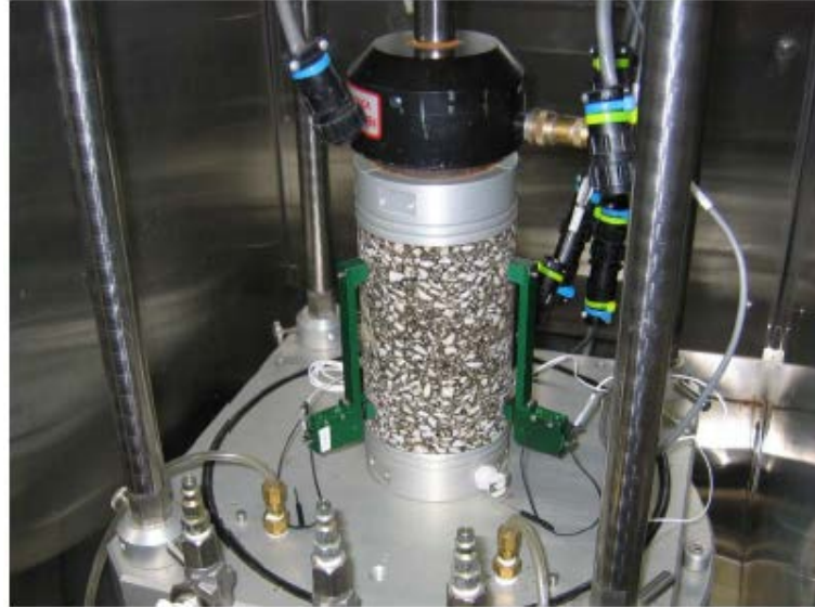
Figure 1. Dynamic modulus testing fixture and setup.
