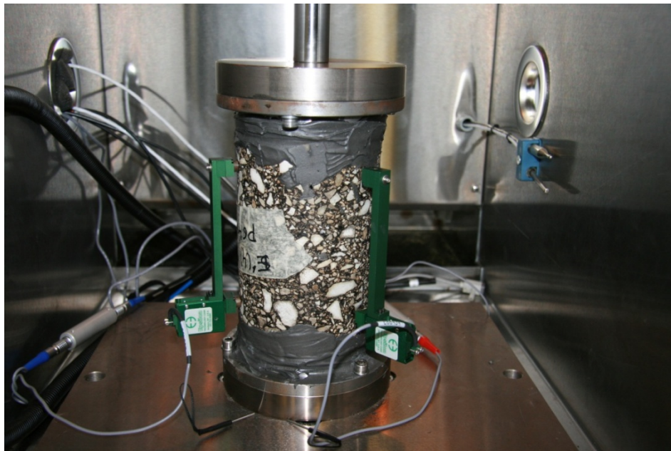
Figure 16. An illustration of the push-pull test fixture and specimen glued to top and bottom plates.
