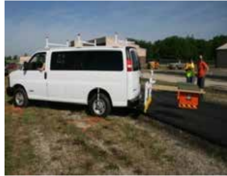
(f) Density measurement using GPR
