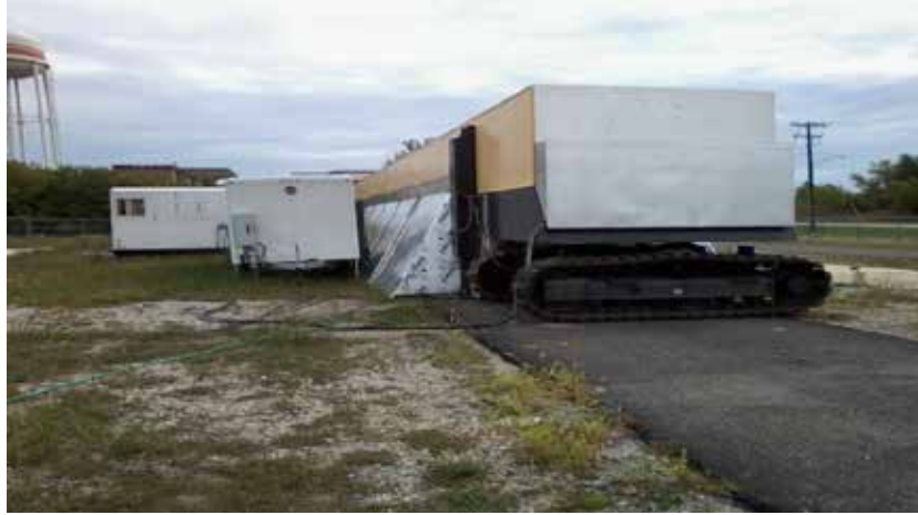
Figure 3.15 In addition to the side panels, heaters were placed around the pavement (Figure 3.6). The main parameters of interest were rutting depth and visual stripping.
