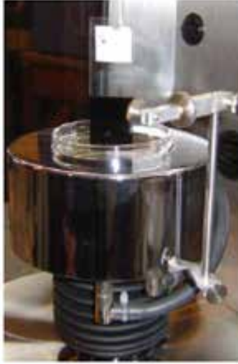
Figure A.1 Dynamic Wilhelmy plate device (Kringos 2007).
