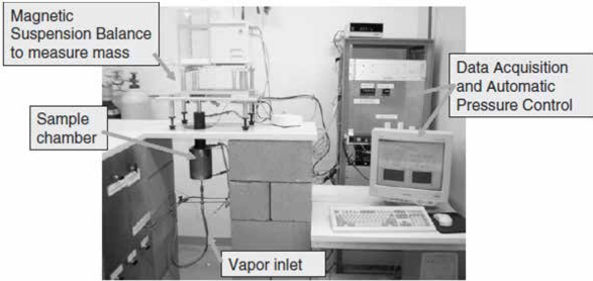
Figure A.3 Universal sorption device (USD) (Bhasin et al. 2007b).
