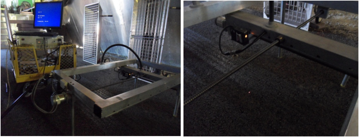
Figure D.10. Rutting measurement using laser technique.
