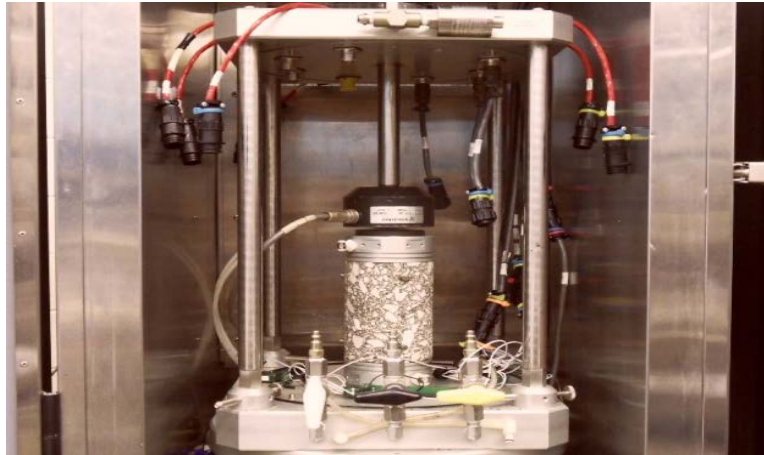
Figure C.2. Test device and setup for complex modulus test.
