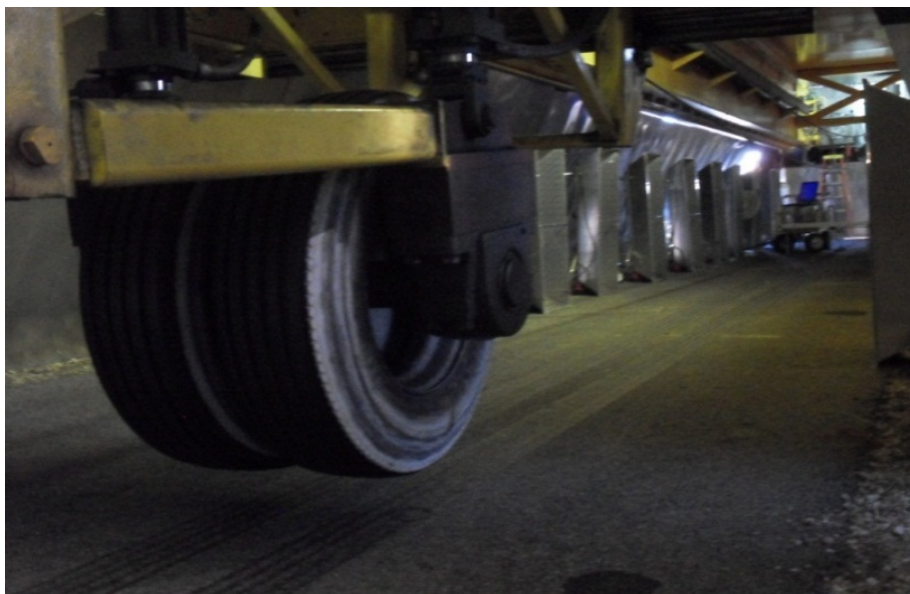
Figure D.9. Dual-tire assembly loading applied 4 ft (1.3 m) from pavement edge.
