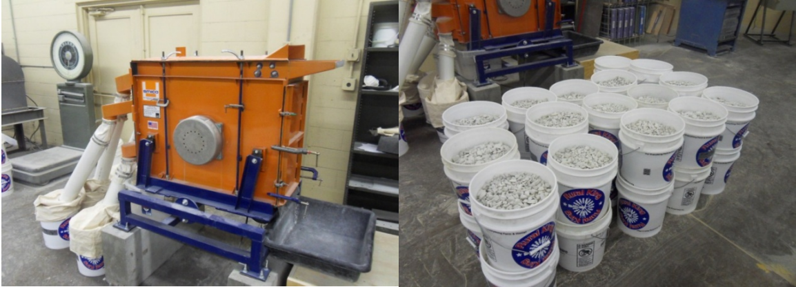
Figure 9. Fractionator (left) and fractionated coarse aggregates (right).
