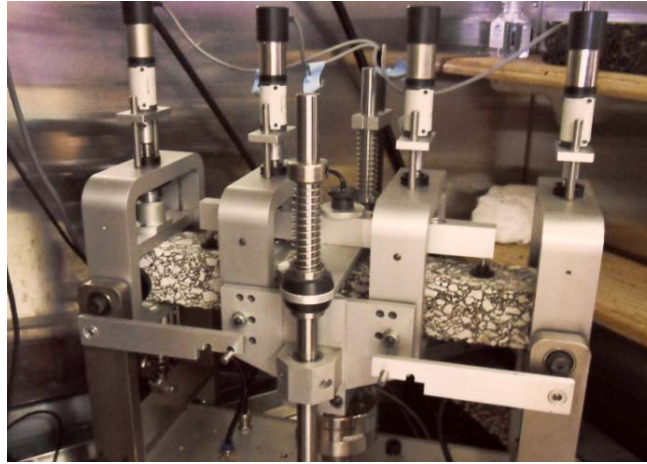
Figure 17. Four-point bending fatigue test device.
