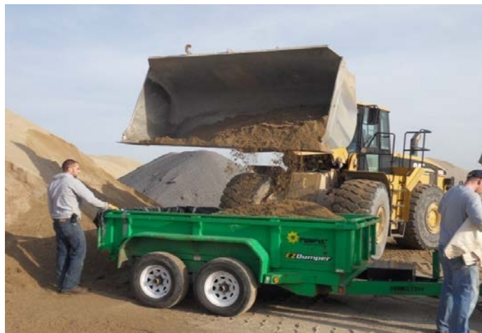
Figure 4. Loading of sampling trailer with bulk aggregate samples.
