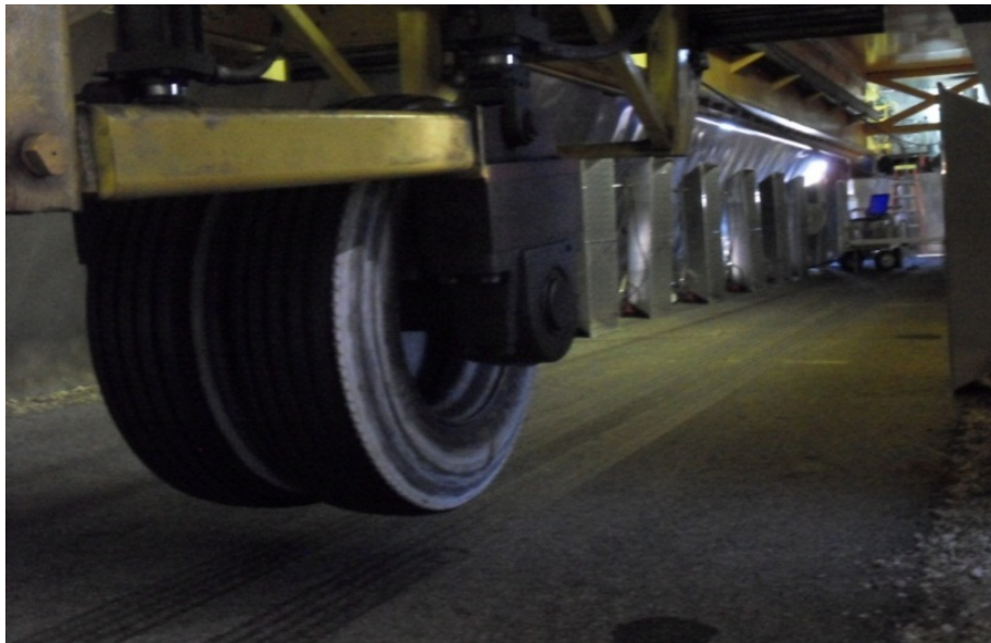
Figure 21. Dual-tire assembly of ATLAS.
