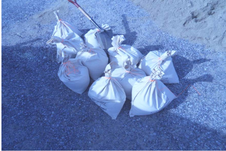
Figure 7. Bagged aggregate samples for physical property testing.
