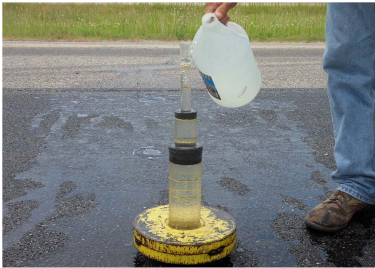
Figure E.1. A falling head permeability test.
