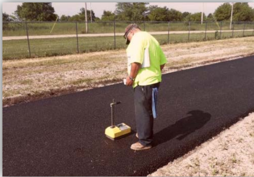
Figure D.8. Nuclear density test (left) and temperature indicator (right).
