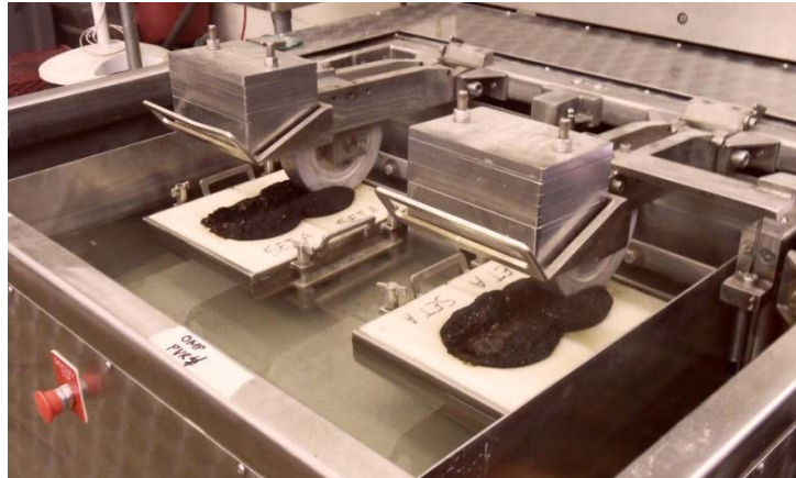
Figure 13. Hamburg wheel tracking device (HWTD) and test setup.
