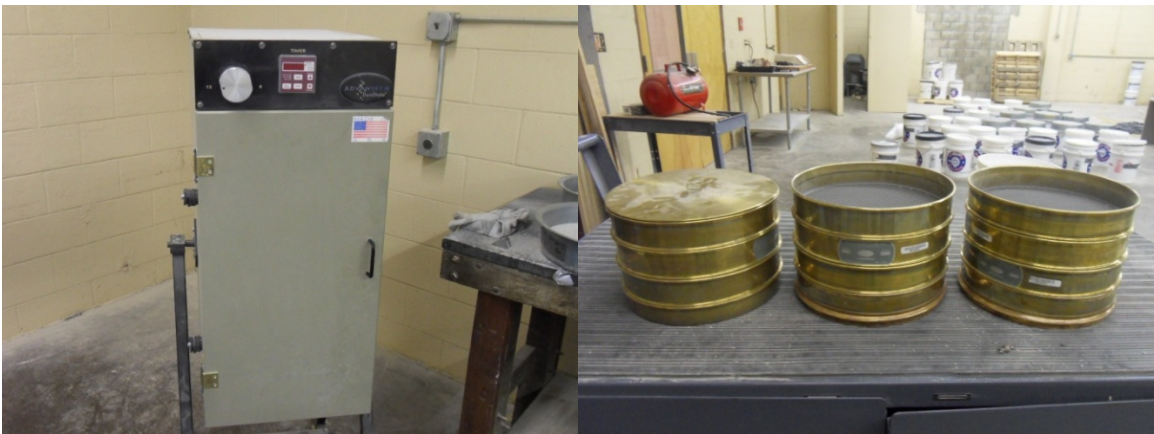
Figure 10. Mary Ann shaker and 12 in diameter sieves used.
