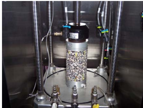
Figure 3.2 Flow number test setup
