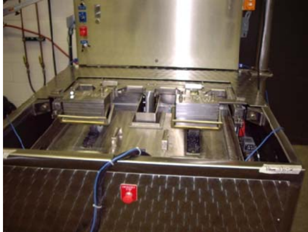
Figure 3.3 Loaded wheel test setup with air condition chamber
