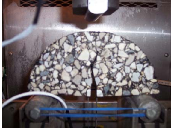
Figure 3.6 Semi-circular beam fracture test setup
