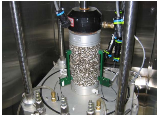
Figure 3.1 Complex (dynamic) modulus test setup
