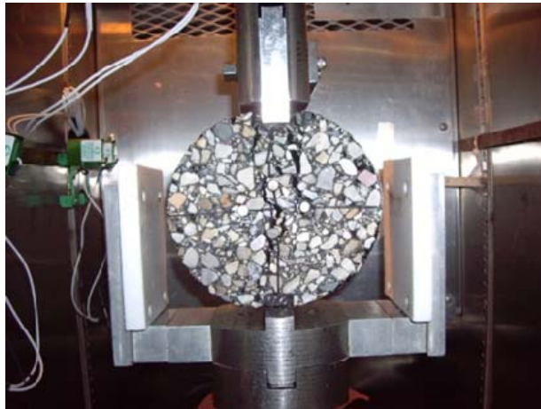
Figure 3.5 Indirect tensile strength test setup
