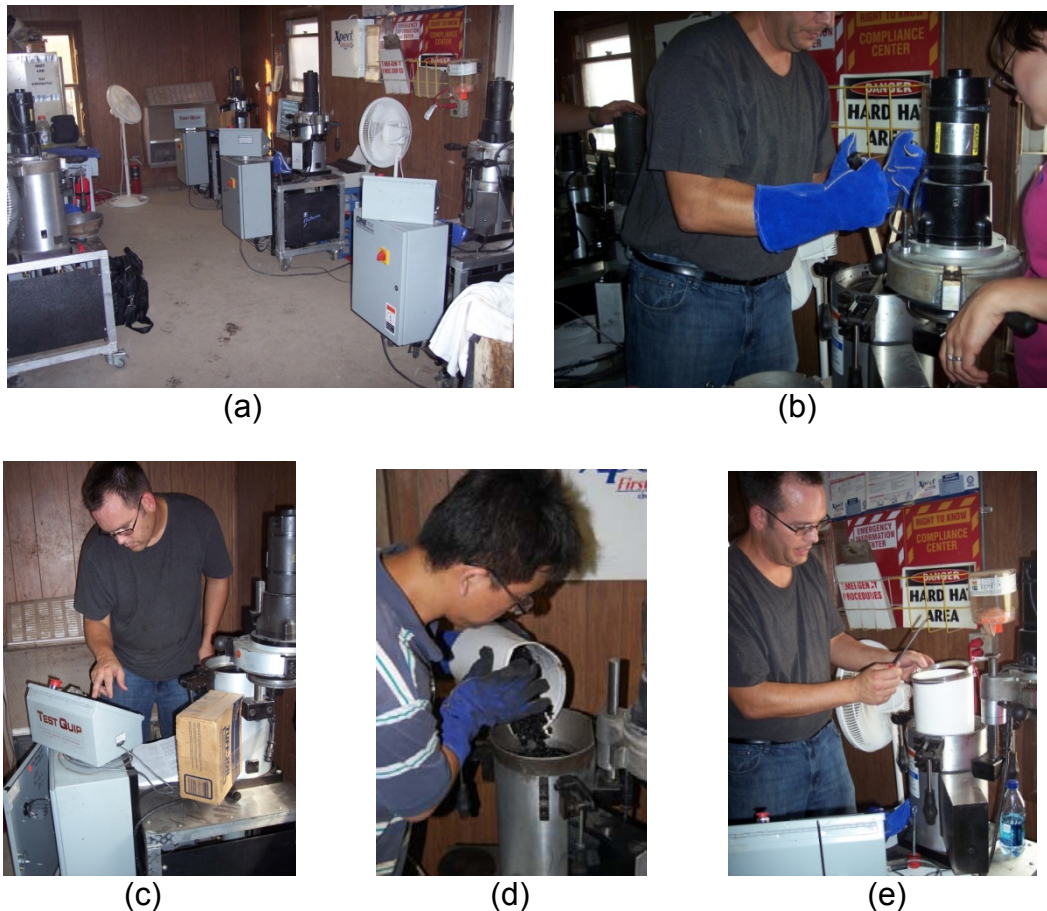
Figure 2.6 Mix compaction process: (a) Gyrotory compactors in the QA lab; (b) Placing the gyrotory mold into the compactor; (c) Setting up the specimen height; (d) Placing loose mix into the gyrotory mold; (e) Protecting gyrotory specimen using a PVC pipe
