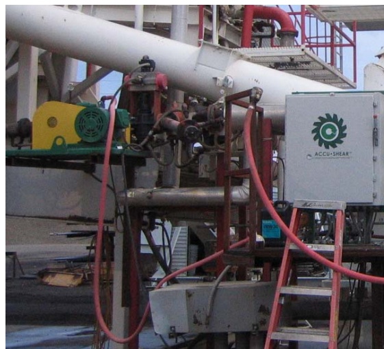
Figure 2.3 Accu-Shear™ technology used for producing foamed asphalt
