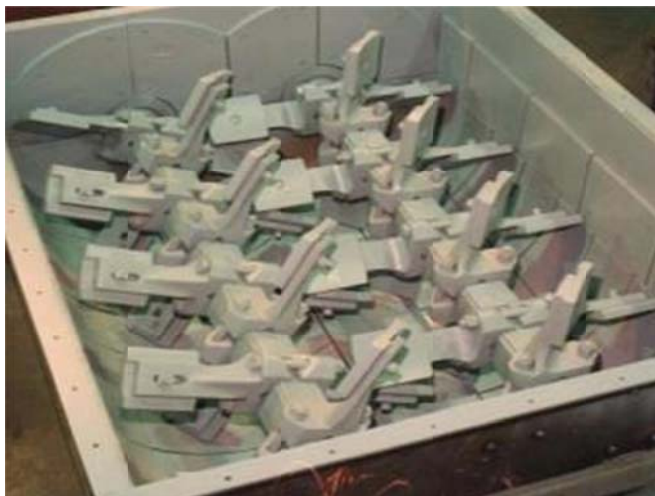
Figure 2.5 Inside of pug mill (NCAT Professors Training Course in Asphalt Technology, 2014).
