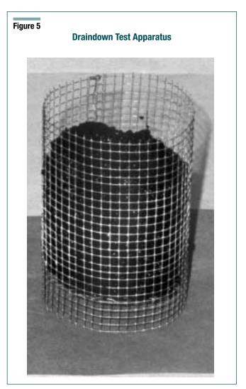
perature, and should meet the criterion in *Tables 4* or *5*. The draindown evaluation at the higher temperatur e (+15°C) provides information as to how sensitive the SMA mixture is to plant temperature fluctuations.
