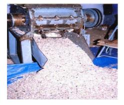
Figure 5: Plastic after passing through shredding machine
