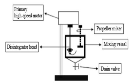
Figure 3: Polymer-bitumen mixing assembly
