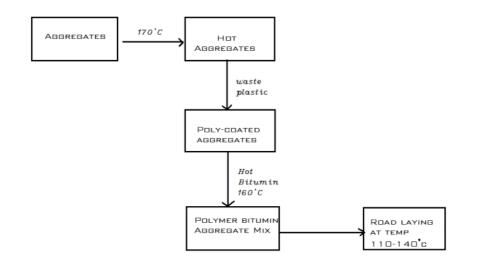
Figure 8: Flow chart of plastic coated bitumen mix from Mir, A. H. (2015)
