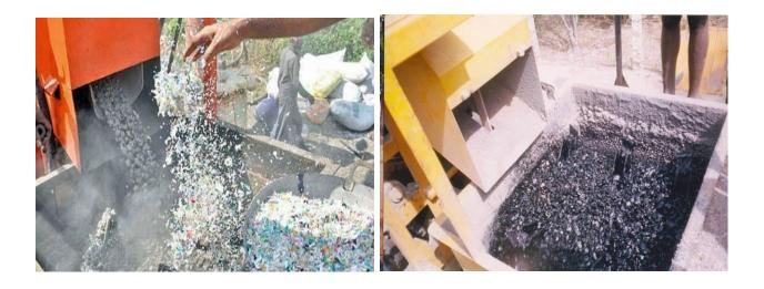
Figure 7: Mixing of plastic and aggregate at mixing chamber from Mir, A. H. (2015) Step 5: The waste plastic coated aggregate is further mixed with hot bitumen and the final mix is used for the construction of the road and the road laying temperature will be between  $110^{\circ}$ C to  $120^{\circ}$ C.
