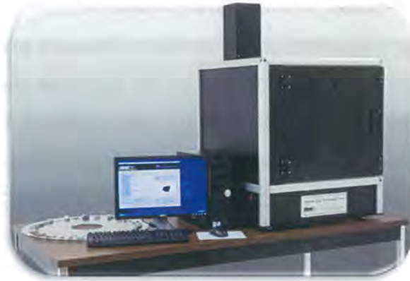
Figure 2. Photo of the exterior of the Pine Instrument's Aggregate Image Measurement System (AIMS) Model AFA2A equipment
