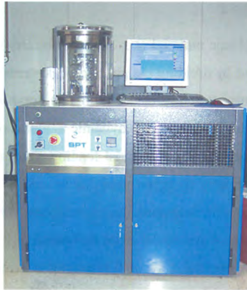
Figure 9. Photo of exterior of the IPC Global's Asphalt Mixture Performance Tester
