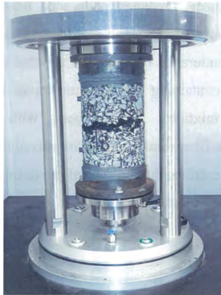
Figure 18. Photo of Failed Sample due to Fatigue Test showing Mid-Specimen Failure
