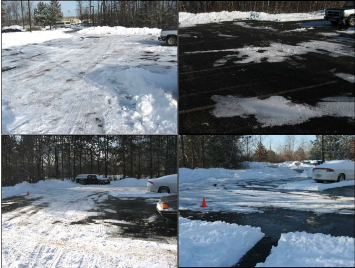
FIGURE 01 Porous asphalt (top) versus standard asphalt (bottom) after one hour and forty minutes (right) (Houle 2010, 1281).
