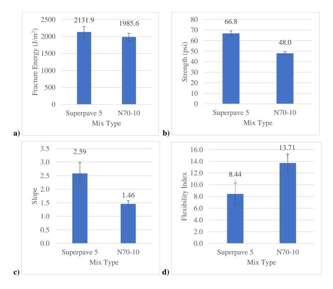
Figure 3. Average IFIT Results a) FE b) Strength c) Slope and d) FI
