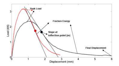
Figure 2. Typical IFIT Output Showing Important Parameters.
